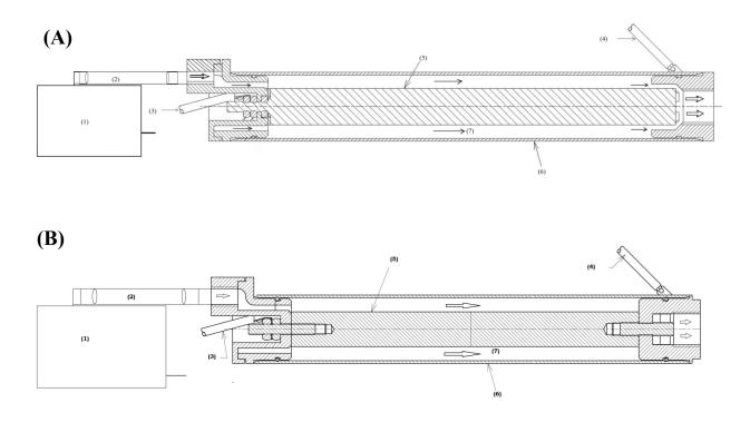
Fig. S1. Simple schematic diagram of the electrode used for electro-degradation.
