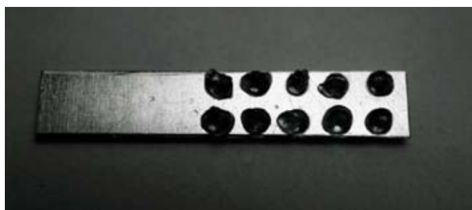
Fig. 1 - Aluminum cryo-plate with embedded shoot tips. Size: 7 mm \times 37 mm \times 0.5 mm with ten wells (diameter 1.5 mm, depth 0.75 mm).
