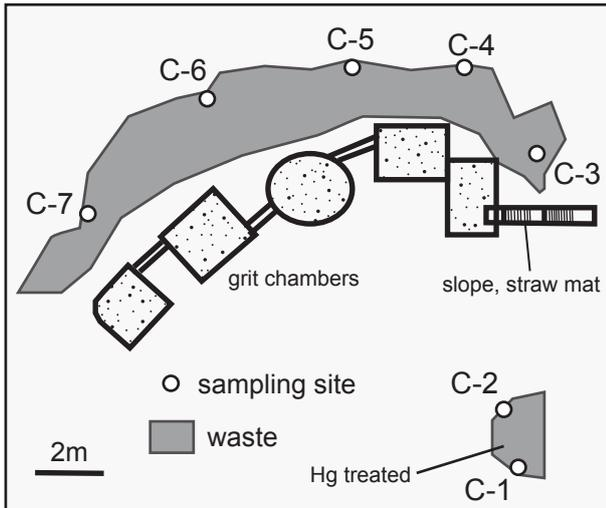
**Fig. 5** Map showing structure of grit chambers and distribution of waste after extraction of gold and auriferous minerals of site C (Fig. 2) at Nzunguni gold mining (Madengi Hill) in central Tanzania.
