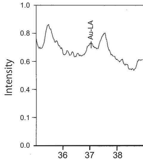
**Fig. 6** Example of XRF qualitative analysis of aurum peak, detected at  $2\theta=36.96^\circ$  from waste sample (A-1) from Nzunguni gold mining (Madengi Hill) in central Tanzania.
