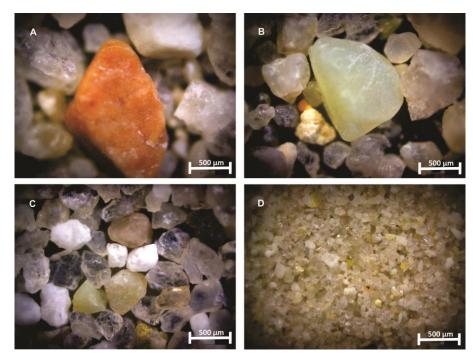
Figure 4.9 Photomicrographs of homogeneous materials of dam mixes *E*, *F*, *G* and *H*.
