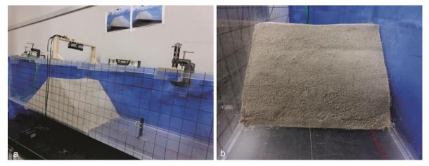
**Figure 4.10 a** Side view of the flume tank. **b** Front view of a dam showing the downstream slope prior to commencement of an experiment.
