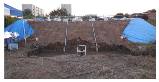
Figure 7.8 Gradual unraveling of the downstream toe under steady-state saturation.
