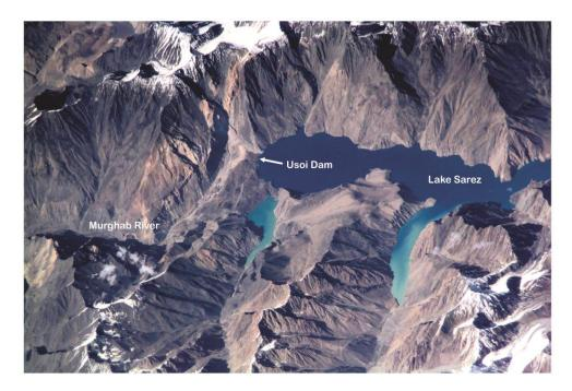
**Figure 2.8** The Usoi natural dam was formed in 1911 by a  $M_w = 7.7 \pm 0.2$  earthquake that triggered a huge rock slide. The rock slide originated as a wedge-like failure and dammed the Murghab River, creating a lake currently known as the Sarez Lake. Several accounts have been given regarding the existence of numerous active seepage holes at the downstream slope (Image: NASA earth observatory file image).
