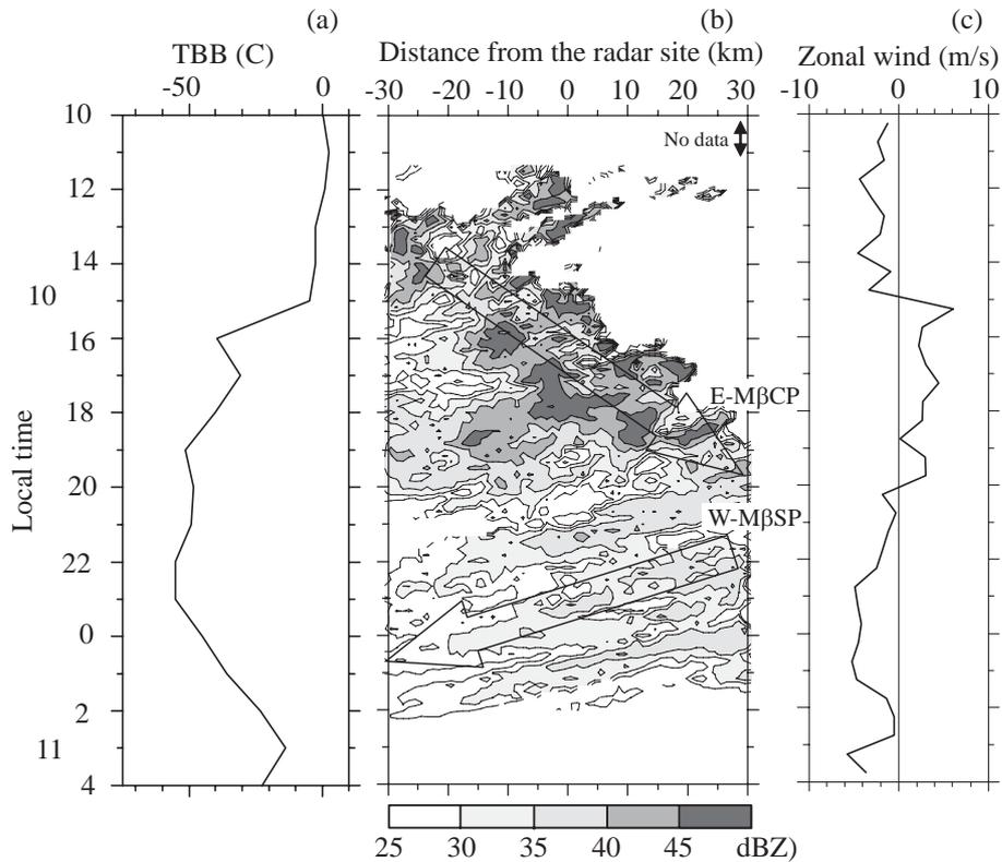
Fig. 6: Time series of (a) 1-hourly pixel TBB data at KT, (b) east-westward maximum CAPPI data over the region extending 15 km north and south of the radar site, and (c) the low-level zonal wind of BLR data averaged over altitudes of 1.4-2.4 km from 10 LST on 10 November to 04 LST on 11 November. The averaged time of zonal wind data is 30 min. The propagations of the E-M $\beta$ CP and W-M $\beta$ SP are indicated by the wide arrow.
