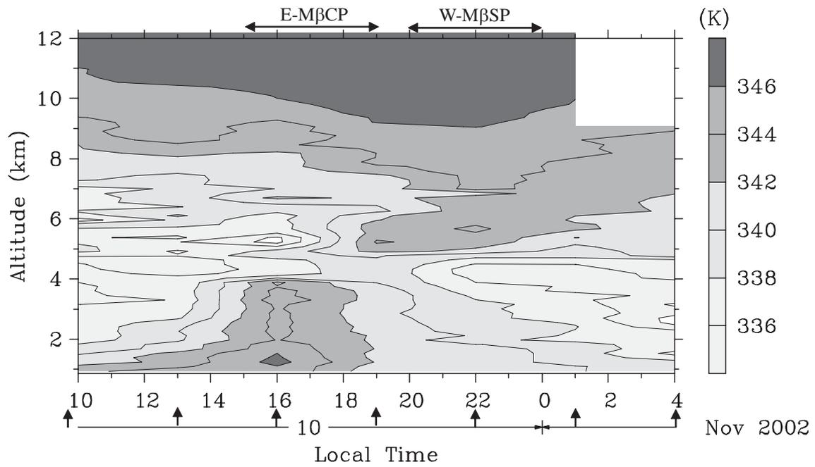
Fig. 8: Time-altitude section of equivalent potential temperature ( $\theta_e$ ) observed by the upper sounding at intervals of 3 hours from 10 LST 10 on November to 04 LST 11 on November. In the bottom of the panel, the observational time of upper sounding is shown by arrows.
