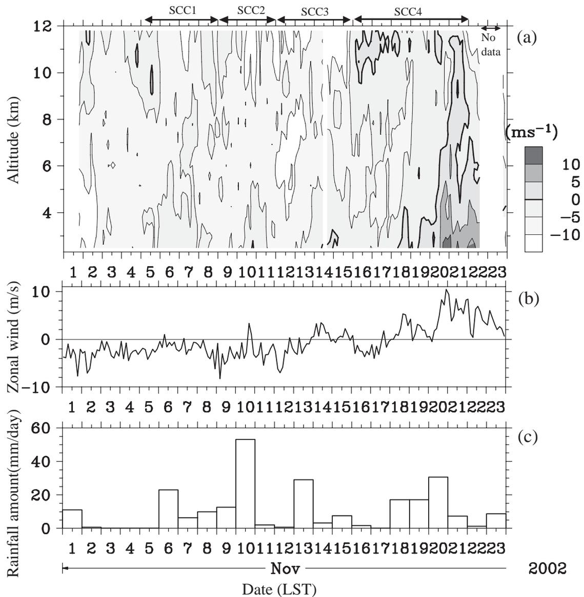
Fig. 3: (a) Time-altitude section of zonal wind observed by EAR, and time series of (b) low-level zonal wind of BLR data averaged at altitudes between 1.4 and 2.4 km, and (c) daily rainfall amount at KT during 01-23 on November 2002. The averaged time of zonal wind data obtained from EAR and BLR is 3 hours.
