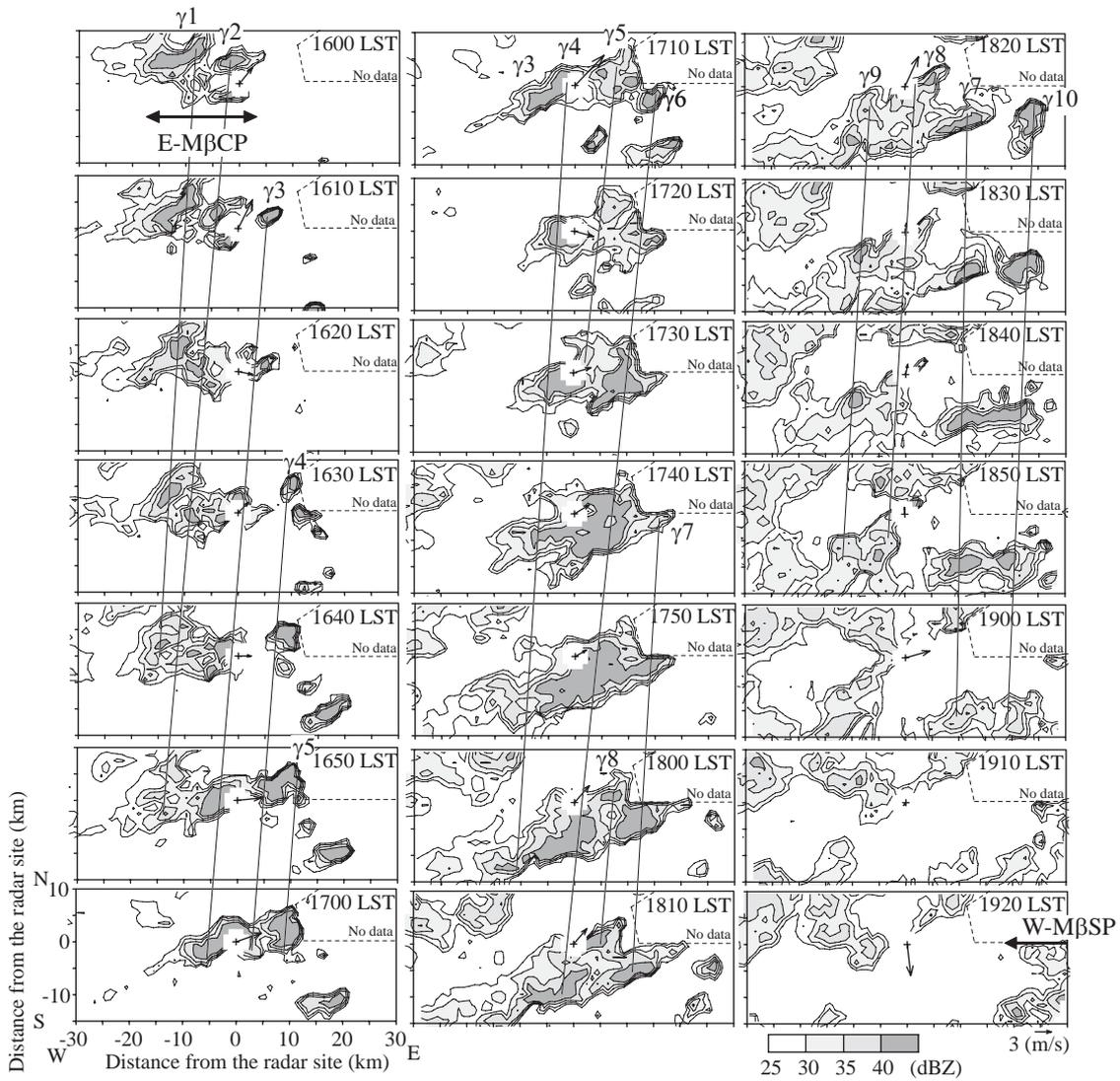
Fig. 9: Horizontal distribution of E-M $\beta$ CP at intervals of 10 min from 1600 to 1920 LST on 10 November. The propagation of M $\gamma$ CPs is indicated by solid lines. The plus mark is the radar site. Arrows shown at the radar site are the low-level wind averaged over altitudes of 1.4-2.4 km from BLR data.
