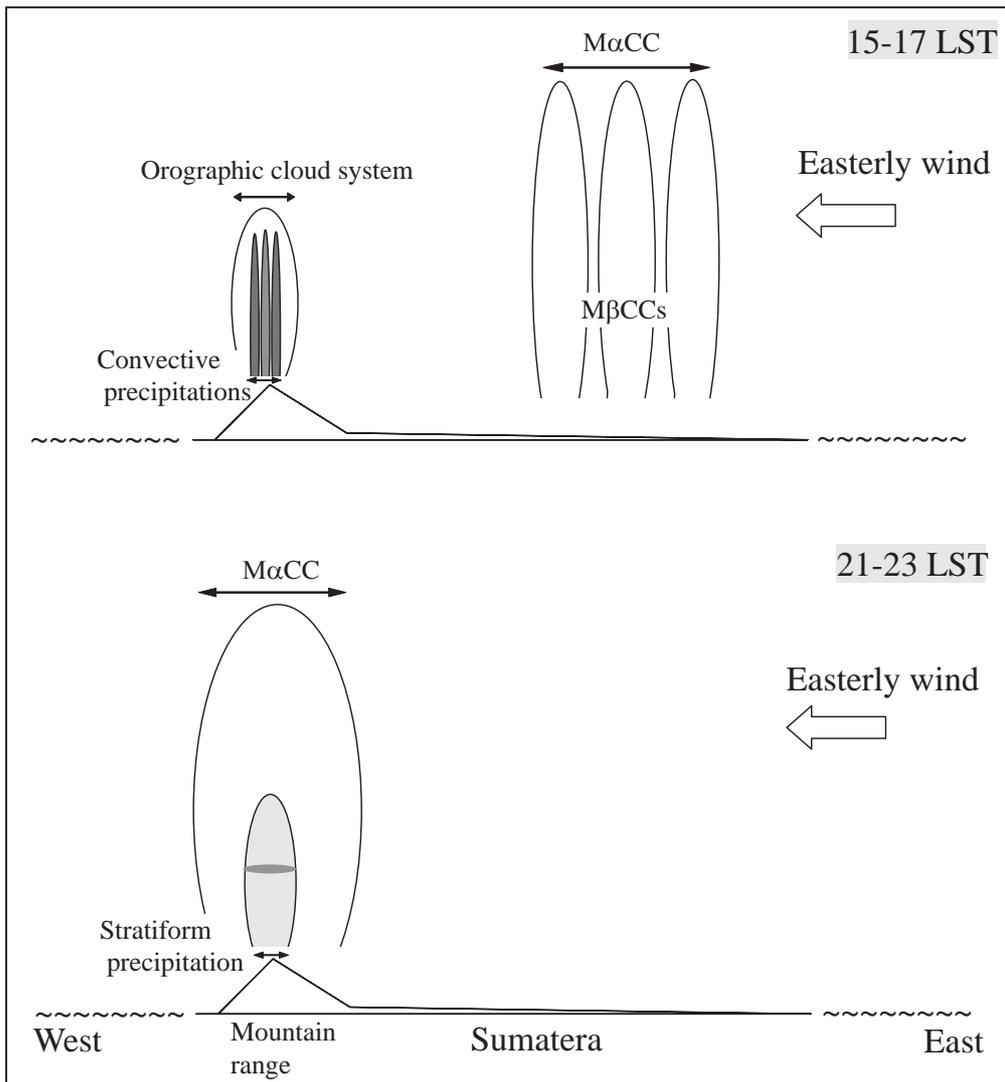
Fig. 12: Schematic illustration of a westward-propagating  $M\alpha$  CC over Sumatra and precipitation systems within an orographic cloud system over the mountain region in western Sumatra.
