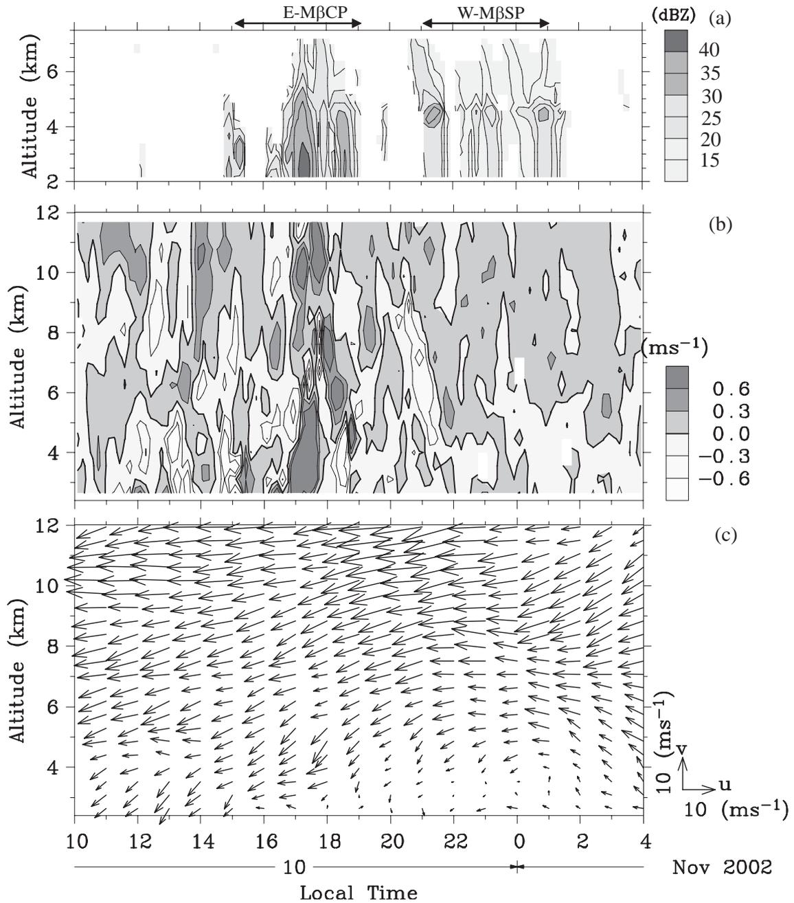
Fig. 7: Time-altitude sections of (a) reflectivity observed by BLR, and (b) vertical velocity and (c) horizontal wind obtained by EAR from 10 LST 10 to 04 LST 11 November. The averaged time of reflectivity and vertical velocity data is 10 min, while that of horizontal wind data is 1 hour.
