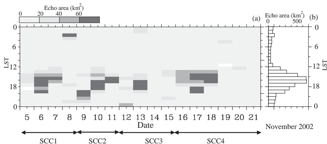
Fig. 11: (a) Local time-day section of intense precipitation echoes ( $\geq 40$  dBZ) averaged at 1-hour intervals from 05 to 21 November. (b) Diurnal variation of echo area summing up the 1-hour interval data during this analysis period. The echo area is calculated over the whole observational area shown by the circle in Fig. 1b.
