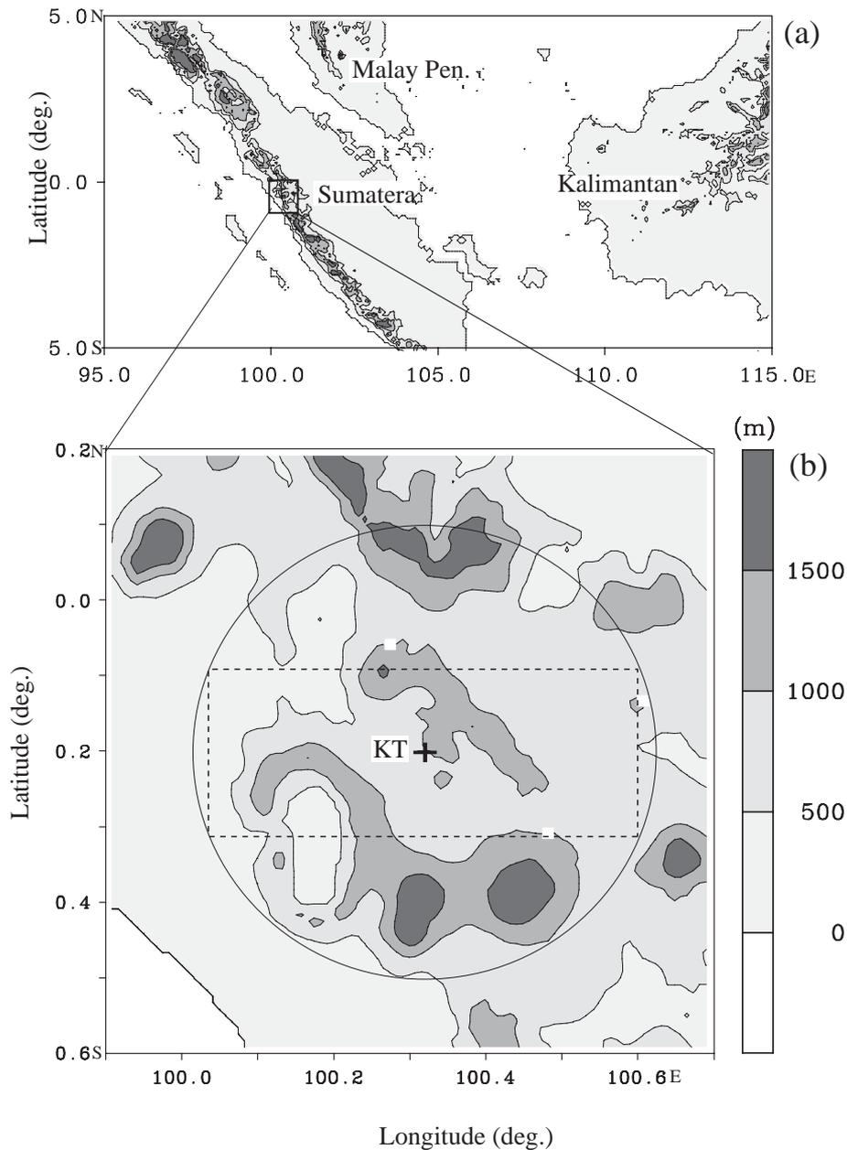
Fig. 1: (a) Surface topography of the Indonesian maritime continent. The map in panel b is magnified from the square area in panel a. A plus mark is the location of the EAR observatory. The circle marks the observational area of the X-band rain radar. The X-band radar data is mainly used in the rectangular area within the circle, because of the orographic shadows surrounding KT.
