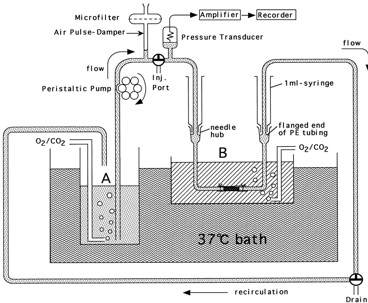
Fig. 1. Diagram of the overall system for squeezed-flow perfusion. Detail explanation is given in the text.
