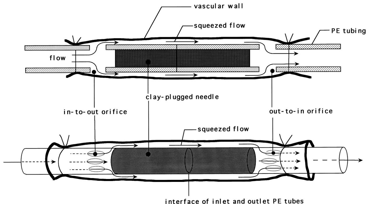
Fig. 2. The core part of the squeezed-flow perfusion system. The upper panel shows the cut view, and the lower panel illustrates the oblique view of the core part of the perfusion system. Detail explanation is given in the text.
