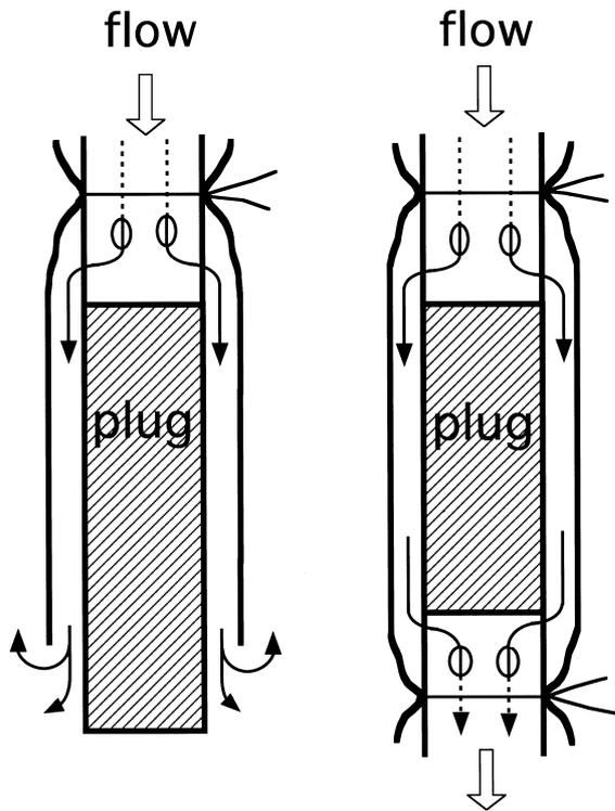
Fig. 5. Comparison of the stainless steel cannula inserting method (left) and the squeezed-flow perfusion method (right). The left panel illustrates the method described in Refs. 7 and 8. The major drawback of their method is that the outflow of the vascular lumen is mixed up with the outer bathing medium, and thus their method is unable to apply a drug exclusively from the intimal side.
