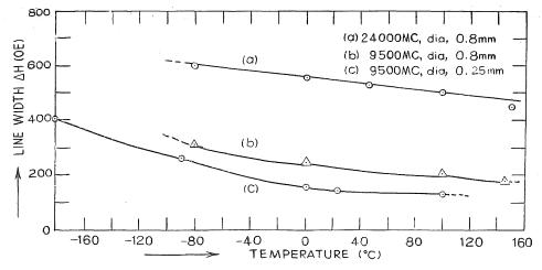
Fig. 3 Temperature dependedce of the line width  $\Delta$ H of Ni<sub>0.7</sub>Cd<sub>0.3</sub>Fe<sub>2</sub>O<sub>4</sub> at 9500 MC and 24000 MC.
