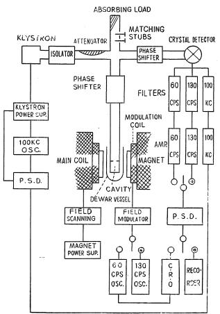
Fig. 1 Block diagram of the appratus at 9500 MC.
