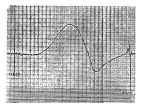
Fig. 2 (a). Derivative curve of resonance line in the mixture of iodine and paraffin.
