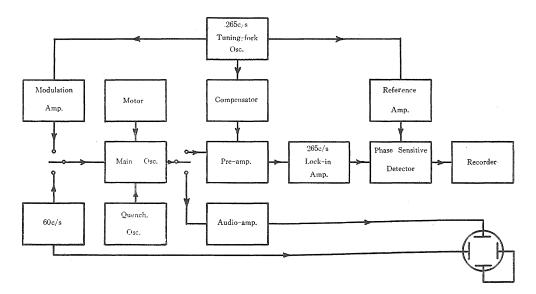
Fig. 1. Block diagram of apparatus.
