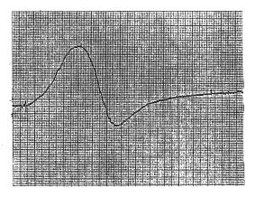
Pig. 2 (c). Derivative curve of resonance line in the irradiated mixture of iodine and paraffin.
