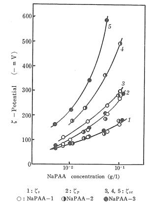
Fig. 1  $\zeta\text{-potential of cotton in NaPAA solutions containing <math display="inline">1\times10^{-5}$  moles/1 potassium chloride.
