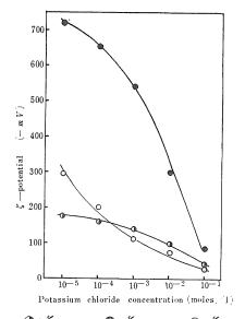
$\textcircled{0}: \zeta_s \qquad \textcircled{0}: \zeta_{sc} \qquad \bigcirc: \zeta_p \\ \mbox{Fig. 2 The effects of potassium chloride on} \\ \mbox{\zeta-potential of cotton in } 0.1018g/1 \mbox{ solution of NaPAA-3.}$
