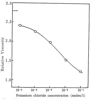
Fig. 4. Plots of viscosity of NaPAA-3 solution against potassium chloride concentration. NaPAA concentration: 0.102g/1 Temperature: 25°C
