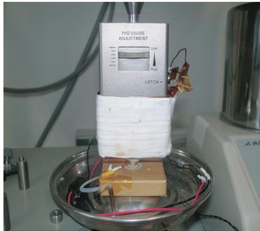
Fig. 2 Teflon sample holder was inserted between the electrodes of the test-fixtured HP16453A, rolled by a heater. Temperature was measured by a thermocouple set near the sample holder.
