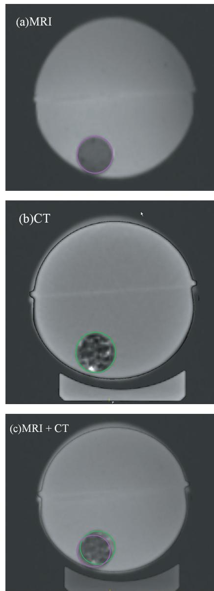
Fig. 5. Image (c) was created by manual fusion of an MR image (a) and a CT scan (b) using software. Distortion of the fused image is obvious, even when the 3 spatial landmarks are matched.
