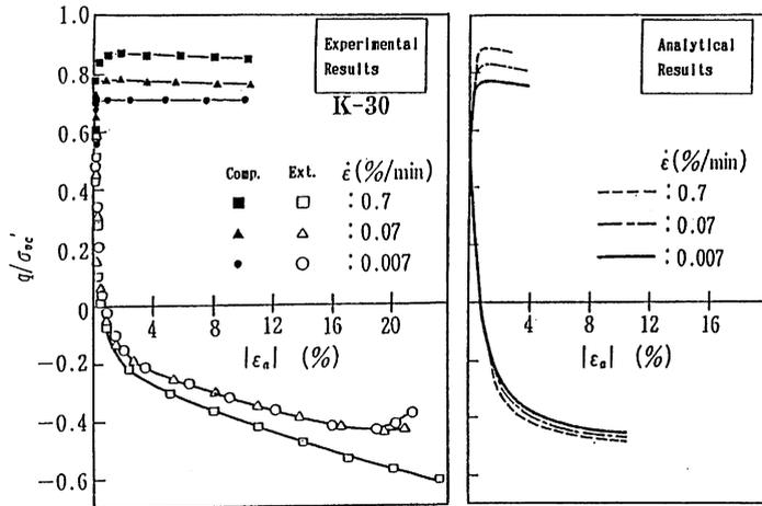
Fig. 1. Comparison of the observed and the computed stress-strain behavior for remolded Kawasaki clay
