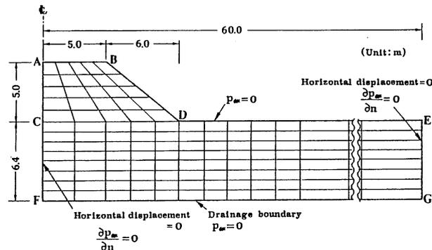
Fig. 5. FEM mesh used in this numerical analysis
