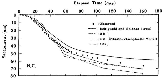
Fig. 8. Case (i): Relationship between the ground surface settlements and elapsed time
