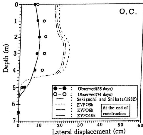
Fig. 12. Case (ii): Distribution of the lateral displacement at embankment toe
