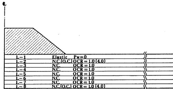
Fig. 6. Model foundation used in this numerical analysis
