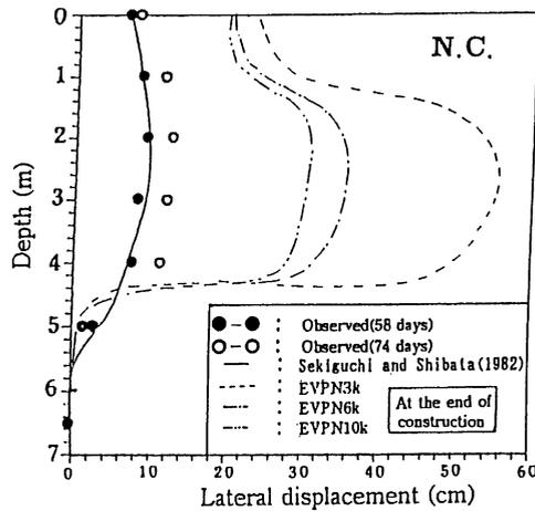
Fig. 9. Case (i): Distribution of the lateral displacement at embankment toe
