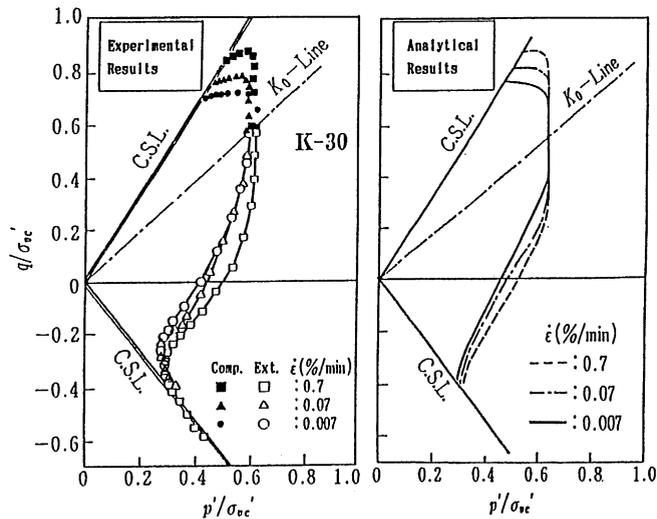
Fig. 2. Comparison of the observed and the computed effective stress paths for remolded Kawasaki clay
