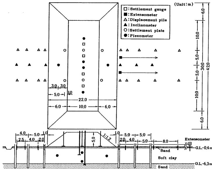
Fig. 3. Plane view and cross-section of Kurashiki Trial Embankment foundation
