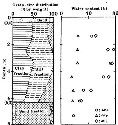
Fig. 4. Soil profile of Kurashiki Trial Embankment foundation
