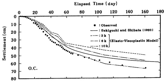
Fig. 11. Case (ii): Relationship between the ground surface settlements and elapsed time
