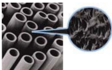
Photo 1 Hollow fiber membranes, in enlarged ( http://www.mrc.co.jp/knowledge/tyukushimaku.html )
