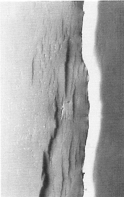
Fig. 3. Fractures developed in Model U. The long side of this photograph is about 5 cm. Note a zigzag pattern of faults which originate in alternative en echelon patterns of right- and left-handed array. This rift consists of a large-normal meandering fault and minor step faults with opposed senses.
