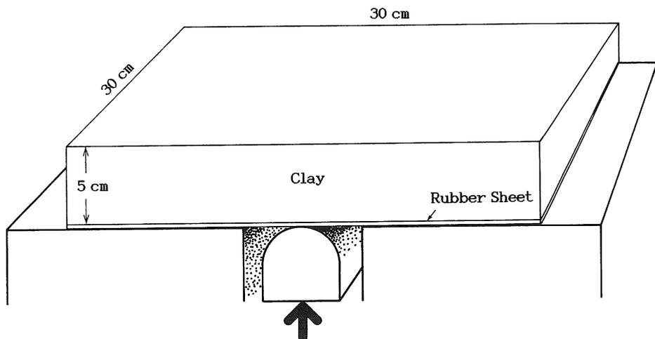
Fig. 1. Simplified sketch of experimental apparatus used for Model U. A motor-driven central block anticlinally pushes up a clay cake (30×30×5 cm) through a rubber sheet.
