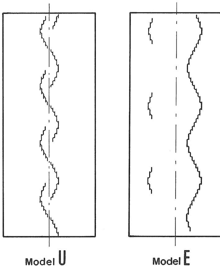
Fig. 9. Simplified patterns of en echelon faults in Model U and E. Sigmoidal faults are arrayed for an echelon of the second order along the rift axis in Model U, whereas only the first order arrangement develops in Model E.
