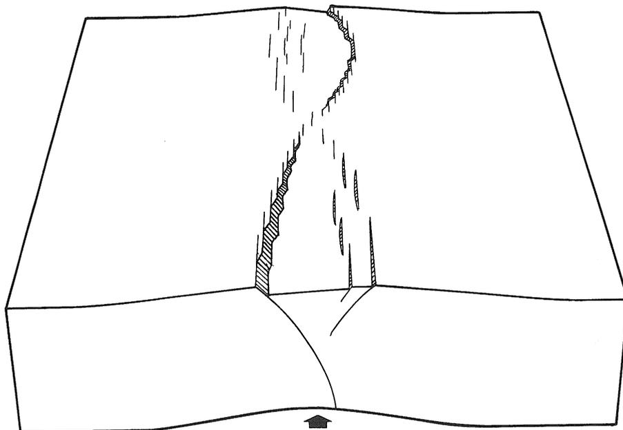
Fig. 6. Schematic illustration of Model U. Short normal faults are arrayed in the first order en echelon arrangement. These faults are linked together to become a sigmoidal major fault, of which sense is reversed across the uplift axis, and of which dip angles show convex-upward.
