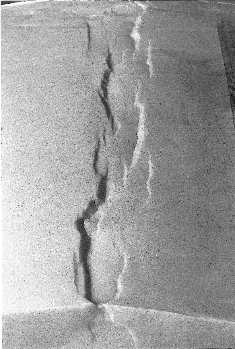
Fig. 5. Model U-2. The uplift rate is  $3.3 \times 10^{-1}$  mm/sec. A quarter wavelength of two sigmoidal faults overlap one another. The width of the rift is variable.
