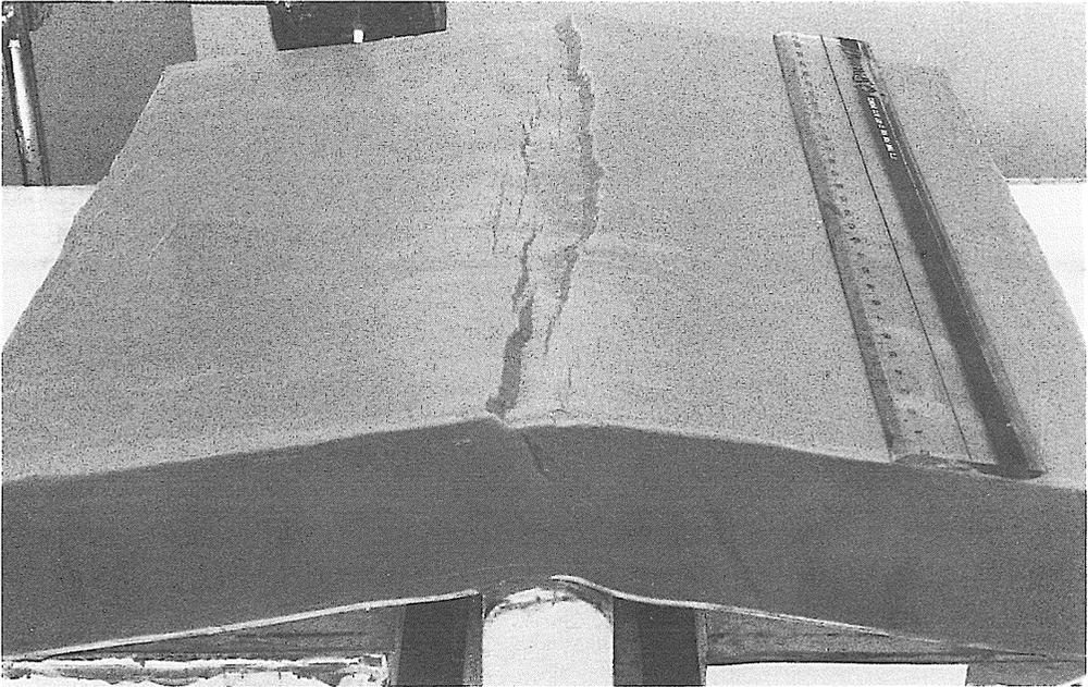
Fig. 4. Model U-1. The uplift rate is  $4.2 \times 10^{-2}$  mm/sec. Fault development is not symmetrical. A normal fault shown in this side crosses the uplift axis and transfers to the fault in the opposite side. Dip angles of the faults are convex-upward.
