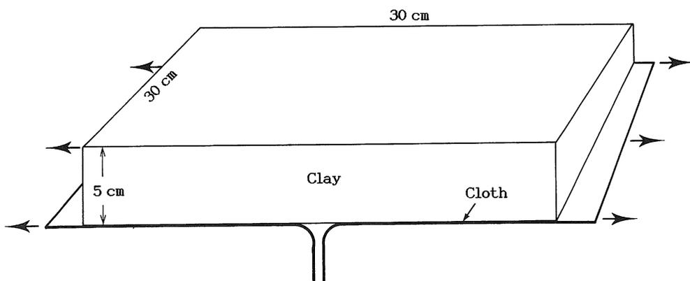
Fig. 2. Simplified sketch of experimental apparatus used for Model E. A clay cake is spread by motor-driven conveyer belts of cloth.
