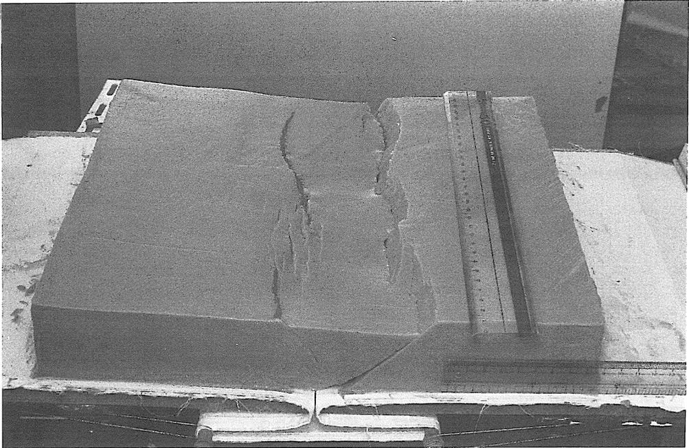
Fig. 7. Model E. The extension rate is  $2 \times (5.0 \times 10^{-3})$  mm/sec. Note a marginal winding fault and step faults. Faults in the vertical side of the model are almost linear or weakly concave-upward.
