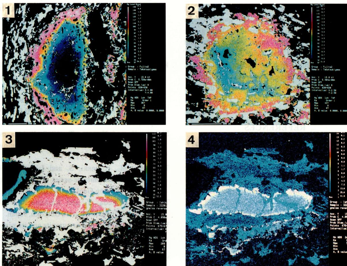
**Fig. 4.** Color maps of element distribution (CMP) within types A, B and C garnets. 1: color map of Mg distribution within type A garnet. Scale bar shows 500  $\mu\text{m}$ . 2: color map of Mg distribution in type B garnet. Scale bar shows 500  $\mu\text{m}$ . 3: color map of Mg distribution in type C garnet. Scale bar shows 200  $\mu\text{m}$ . 4: color map of Mn distribution in type C garnet.
