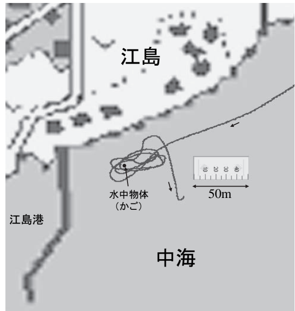
図4. 水中物体の探索実験の航跡図 Fig. 4. Surveyed route of the search experiment of the submerged object.
