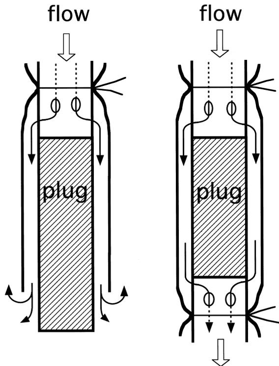
Fig. 5. Comparison of the stainless steel cannula inserting method (left) and the squeezed-flow perfusion method (right). The left panel illustrates the method described in Refs. 7 and 8. The major drawback of their method is that the outflow of the vascular lumen is mixed up with the outer bathing medium, and thus their method is unable to apply a drug exclusively from the intimal side.
