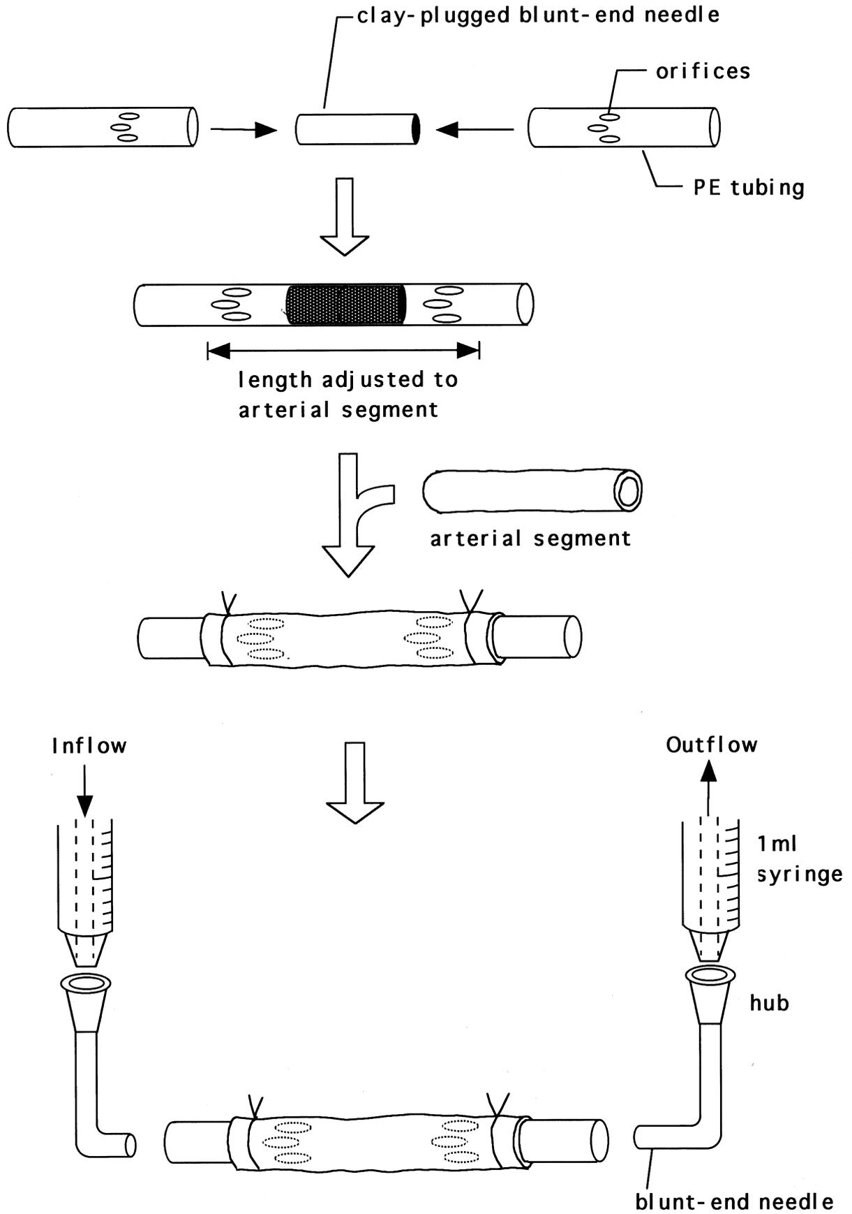
Fig. 3. Step-by-step procedures for setting up the vascular segment. Detail is explained in the text. See the section "How to set a vessel segment to the squeezed-flow system."
