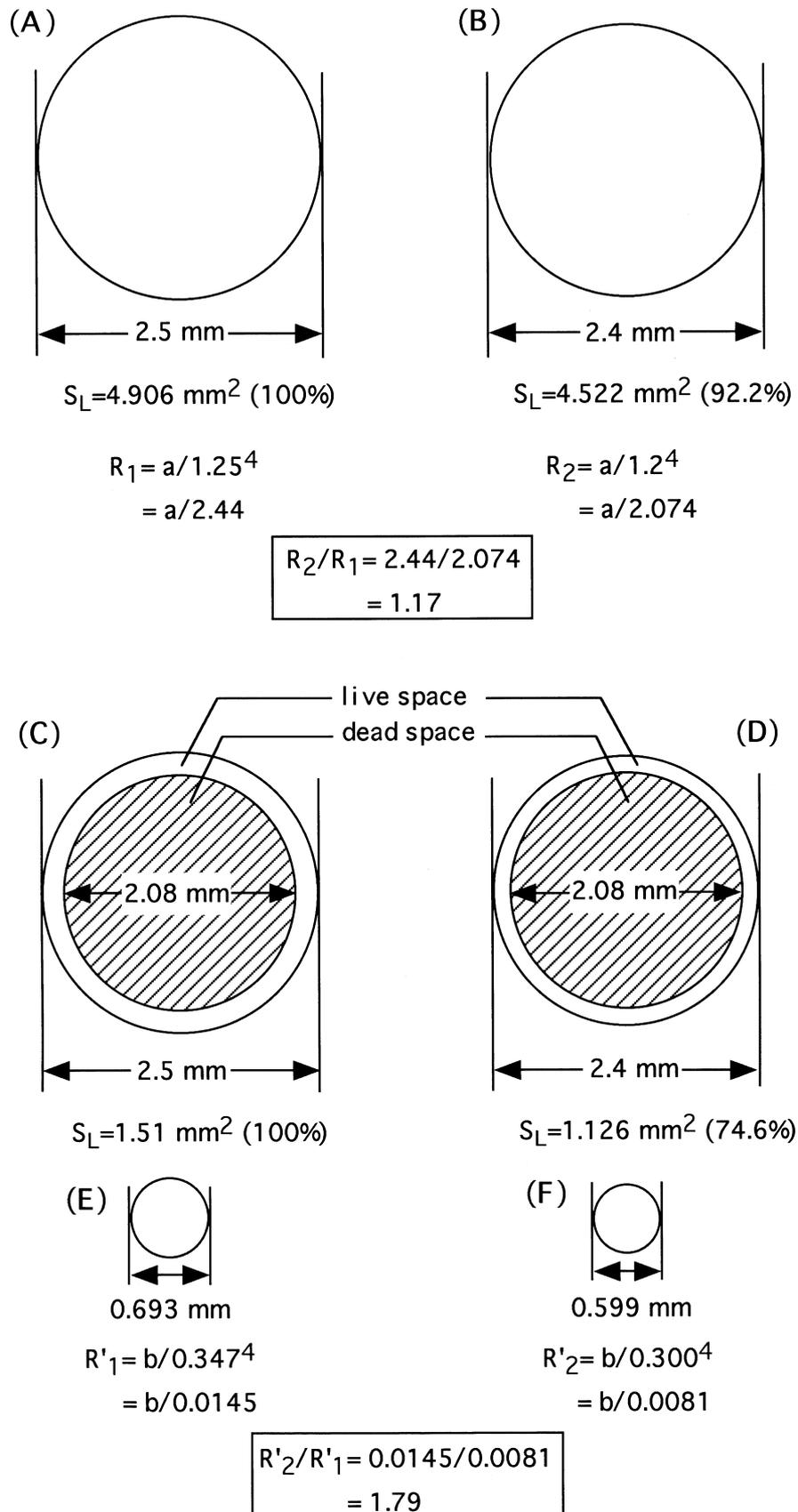
Fig. 4. Examples of calculation in application of the Poiseuille's law. See the text for detail explanation.  $S_L$ : cross-sectional area of the live (effective) vascular lumen space through which the perfusate flows.  $R_1$ ,  $R'_1$ ,  $R_2$ , and  $R'_2$ : resistance against the constant flow.  $a$  and  $b$ : constants derived from Poiseuille's equation.
