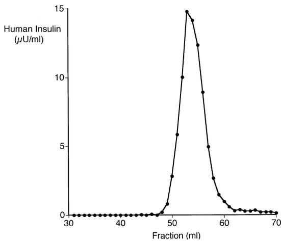
Fig. 4. Gel filtration pattern of recombinant human insulin. Samples of 500 μl were applied on a Sephadex G-50 column (1.0 x 100 cm). The volume of each fraction was 1.0 ml.
