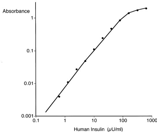
Fig. 3. A representative standard curve of the sandwich enzyme immunoassay of polystyrene plate method for human insulin.
