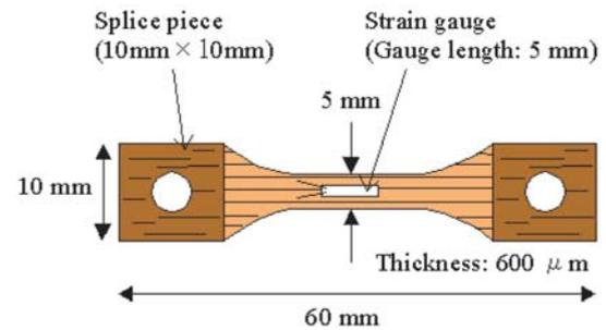
(b) Specimen used for uniaxial tensile test.
