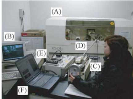
Fig. 3. System used for the X-ray stress analysis. Legend: (A) X-ray diffraction equipment, (B) Personal computer for controlling (A), (C) Loading device (material-testing machine), (D) Bar for applying compressive load to jig, (E) Data acquisition controller, (F) Personal computer for storing the experimental data.
