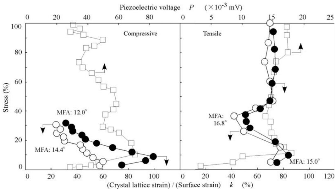
Fig. 4. Relationships between the ratios of the crystal lattice strain to the surface strain, the piezoelectric voltage, and the stresses. Legend: Arrows show the horizontal axis of each curve, MFA: Microfibril angle. Note: The stress values depicted in the vertical lines are given as the percentage of the breaking stress.
