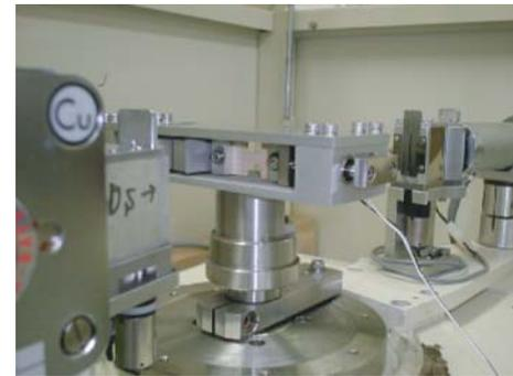
(b) The jig installed in the X-ray diffractometer.
