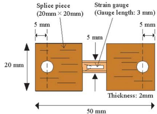
(a) Specimen used for uniaxial compressive test.
