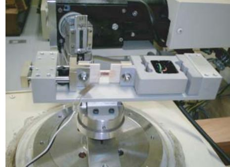
(a) The jig used to apply compressive stress to the specimen.
