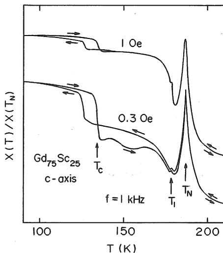
Fig. 5. Low isofield a-c susceptibility normalized by the each value of  $T_N$  for decreasing and increasing temperature.
