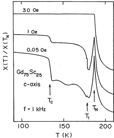
Fig. 4. Low isofield  $a$ - $c$  susceptibility normalized by the each value of  $T_N$  vs temperature for  $Gd_{75}Sc_{25}$  along the  $c$ -axis.
