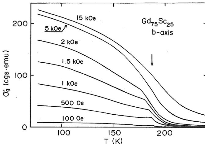
Fig. 1. Isofield magnetization vs temperature for  $Gd_{75}Sc_{25}$  along the *b*-axis.
