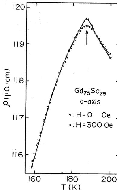
Fig. 6. Electrical resistivity vs temperature for  $Gd_{75}Sc_{25}$  along the  $c$ -axis. Open circles represent the magnetoresistance in the field at 300 Oe along the current direction.
