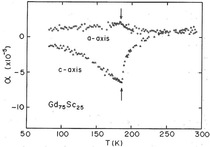
Fig. 8. The thermal expansion coefficients measured along the  $a$ - and  $c$ -axes as function of temperature.
