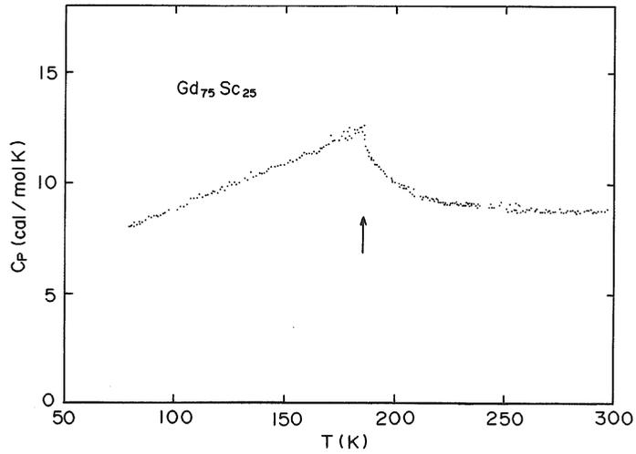
Fig. 9. Specific-heat vs temperature for  $Gd_{75}Sc_{25}$  alloy.
