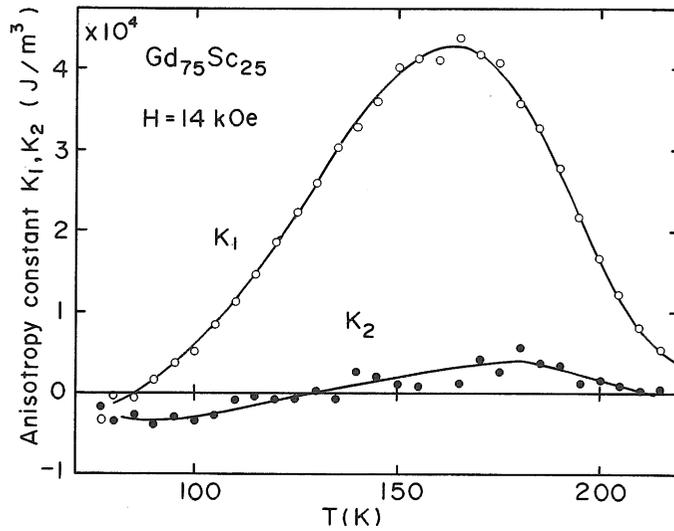
Fig. 10. A plot of anisotropy constants  $K_1$  and  $K_2$  vs temperature.
