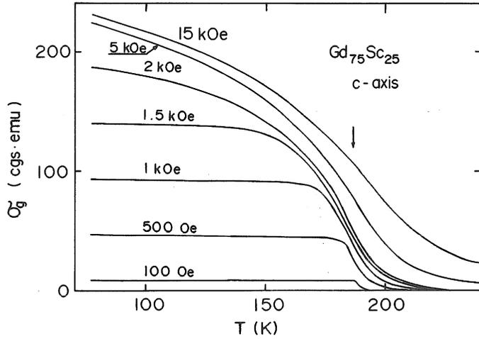
Fig. 2. Isofield magnetization vs temperature for  $Gd_{75}Sc_{25}$  along the  $c$ -axis.
