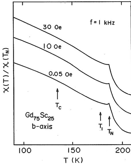
Fig. 3. Low isofield  $a$ - $c$  susceptibility normalized by the each value of  $T_N$  vs temperature for  $Gd_{75}Sc_{25}$  along the  $b$ -axis.
