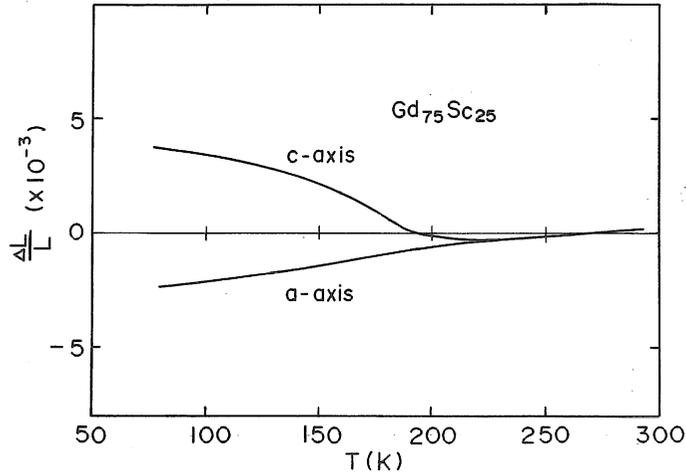
Fig. 7. The thermal expansion measured along the  $a$ - and  $c$ -axes as a function of temperature.
