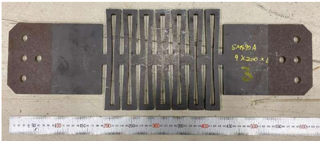
Photo 3.5. F1-1 Model after compression experimental tests.
