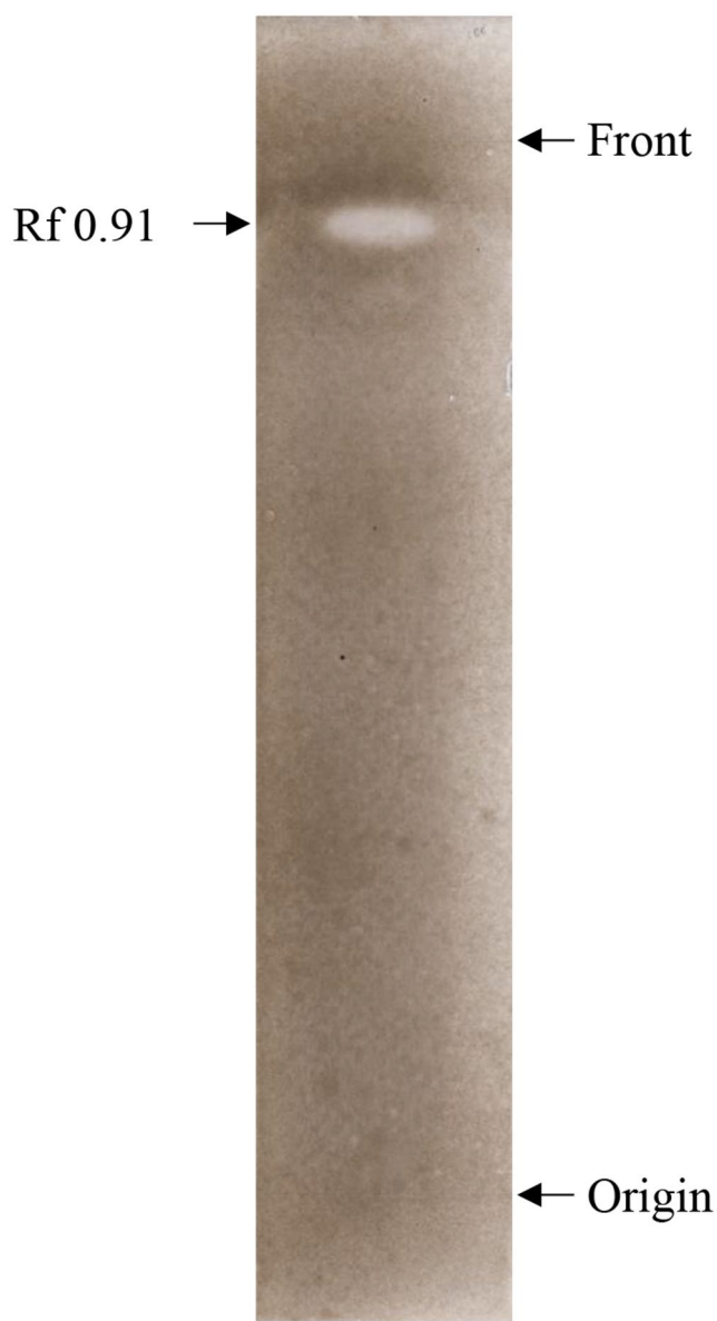
Fig. 2 Thin-layer-chromatography (TLC) bioassay to detect antifungal activity of traversianal against Pyricularia oryzae . Silica gel TLC plate was spotted with traversianal at 30 ppm (100 \mu l) and developed in chloroform–ethanol–water (40:10:1, v/v/v), then sprayed with molten potato sucrose agar containing >1.0 \times 10^7 conidia/ml and incubated at 25 \pm 2 °C for 7 days
