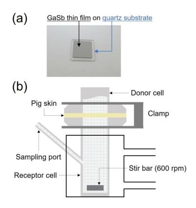
**Fig. 1.** (a) GaSb thin film on a quartz substrate. (b) Franz diffusion cell for experiments *in vitro*.
