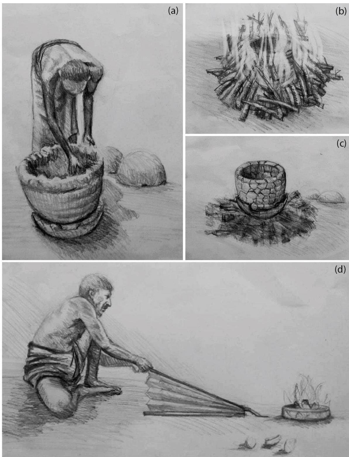
Fig. 6.1. Steps to make a crucible-shaped steel furnace until activated. (a) Crucible-shaped furnaces are made on the ground using clay pieces. They may use a rounded fragmented earthenware base for making the rounded crucible base (b) Open firing the Crucible Furnace structure on the ground (c) Cracked furnace structure after the open firing process (d) Furnace activated by the bellow method after re-built furnace fragments in a pit (Drawn by Nalin Jayarathna) (after Wijepala, S M Young and Ishiga, 2022).
