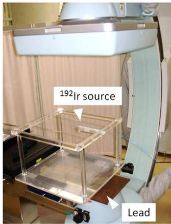
**Figure 5.** Configuration of the weekly linearity measurement of  $[\gamma]$ . A source was placed at rotation center (isocenter) of the C-arm on an acrylic box. For acquisition of the image solely by gamma-rays, dummy X-rays were emitted while shielding the X-ray generator with a lead plate.
