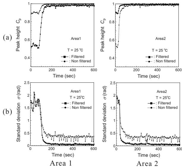
**Fig. 4** Time dependence of (a) peak value of cross-correlation function  $C_p$  and (b) standard deviation of phase difference  $\sigma$  in the different areas of 1 and 2 in Fig. 3.
