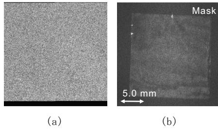
**Fig. 2** Images of (a) the hologram and (b) the reconstructed intensity images of a painted surface.
