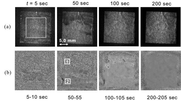
**Fig. 3** Reconstructed intensity and phase difference images of the aluminum surface painted with silver paint varied with time: (a) intensity image and (b) phase difference image between adjacent frames.
