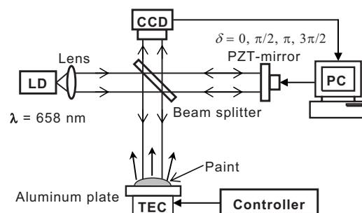
**Fig. 1** Experimental setup: LD, laser diode; CCD, charge-coupled device; PC, personal computer; and TEC, thermoelectric cooler.
