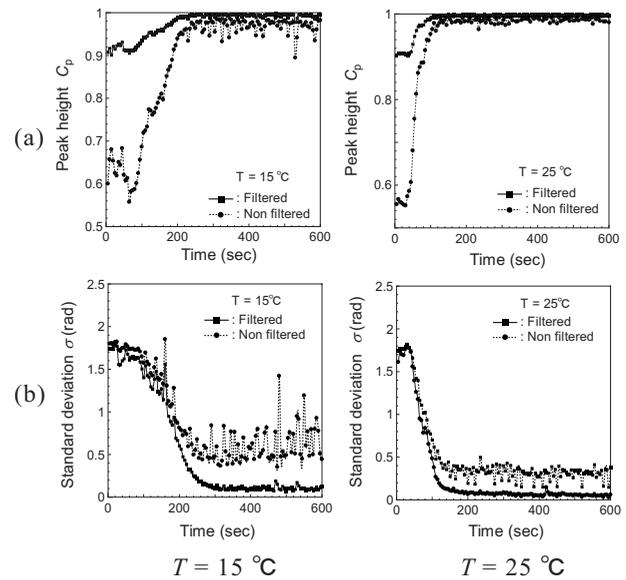
**Fig. 5** Temperature dependence of variation in the values of (a) cross-correlation  $C_p$  and (b) standard deviation of phase difference  $\sigma$ .
