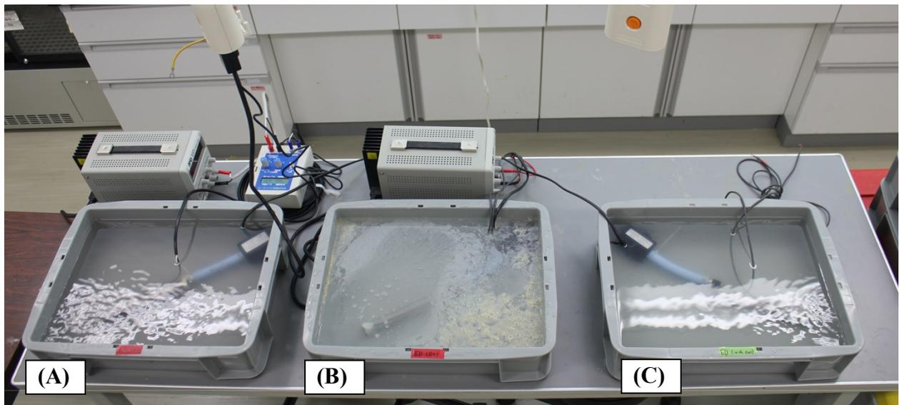
**Fig. S2.** Electro-degradations of nutrient solution following without plant experiment for 24 hours. (A) AC-ED was applied at 50% duty ratio, 2.0 amperes alternate current, and 14.0 volts. (B) The DC-ED was applied at 2.0 ampere and 18.0 volts. (C) Control- without ED application, nutrient solution was flowed using pump only. (Experiment II)
