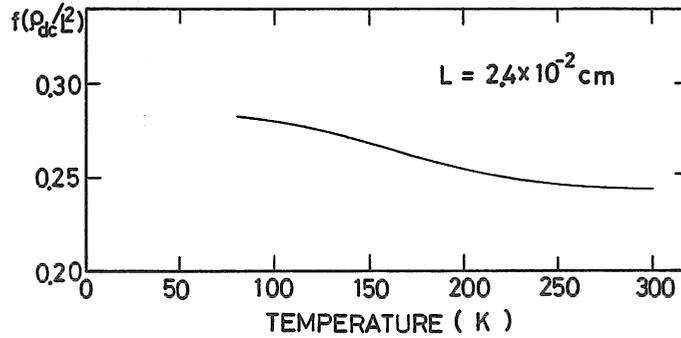
Fig. 7. The temperature dependence of  $f(\rho_r/L^2)$  evaluated by assuming  $\rho_r = \rho_{dc}$ .
