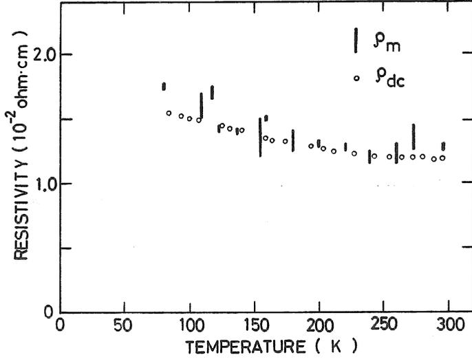
Fig. 6. Microwave resistivities of Si single crystal as a function of temperatures.
