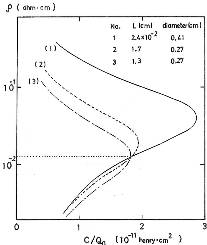
Fig. 5. The  $\rho$  vs.  $C/Q_0$  curves obtained at 300 K with disk-type samples of Si of  $\rho_{dc} = 1.2 \times 10^{-2} \Omega \text{ cm}$  (300 K).
