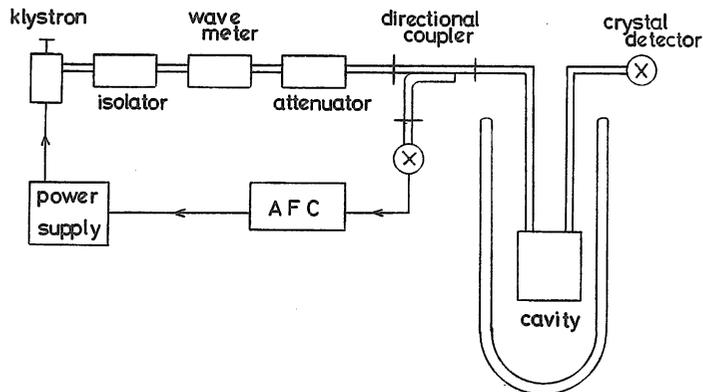
Fig. 3. The blockdiagram of the microwave system.
