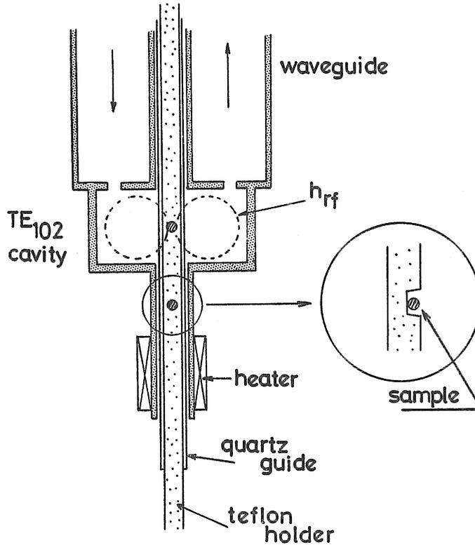
Fig. 4. Rectangular  $TE_{102}$  microwave cavity.
