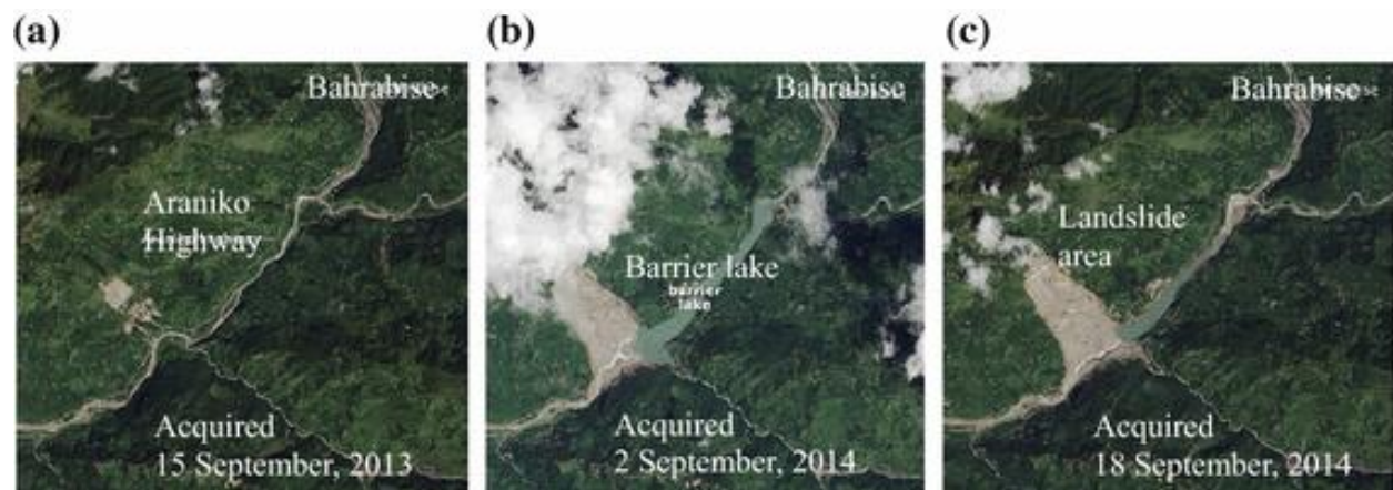
Fig. 2.3 Landsat 8 satellite images a) before landslide; b) after landslide and before landslide dam breach; and c) after landslide dam breach (Shrestha and Nakagawa, 2016).
