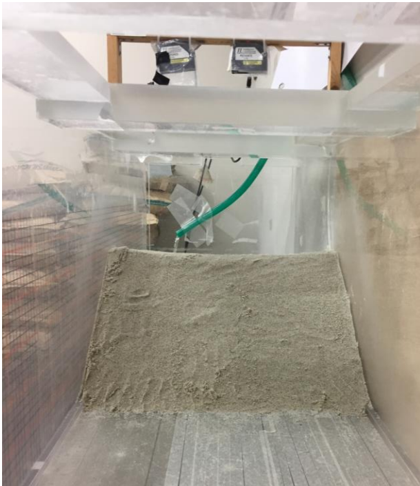
Fig. 8.4 Photographs of experimental setup. a) Side view of flume tank during experiment; b) Downstream slope of dam with laser sensor at the top of flume tank
