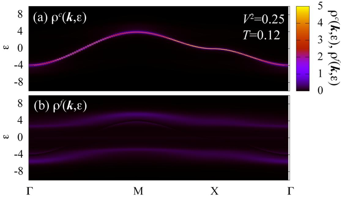
**Fig. 10.** (Color online) (a) Conduction-electron component  $\rho^c(\mathbf{k}, \epsilon)$  and (b)  $f$ -electron component  $\rho^f(\mathbf{k}, \epsilon)$  of the spectral functions along the symmetric line in the first Brillouin zone for  $V^2 = 0.25$ ,  $U = 8$ , and  $\alpha = 0.5$  at  $T = 0.12$ .
