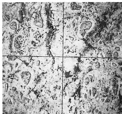
Fig. 3. Photomicrograph of serpentinitized saxonite (T-5).
