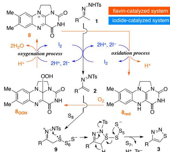
**Scheme 3. Proposed Mechanism for the Flavin-Iodine-Catalyzed Aerobic 1,2,3-Thiadiazole Ring Formation**
