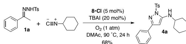
**Scheme 4. Flavin-Iodine-Catalyzed Aerobic Cross-Coupling of **1a** and Isocyanide**
