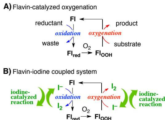
**Scheme 1.** Flavin-Catalyzed (A) Aerobic Oxygenation of Substrate Using Reductant and (B) Aerobic Oxidative Transformation of  $\text{I}^-$  to  $\text{I}_2$
