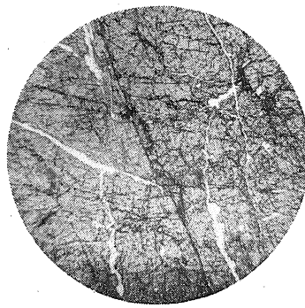
Fig.9 Massive chromite with fractures filled by serpentine. X23 South No.5 deposit of Wakamatsu mine.
