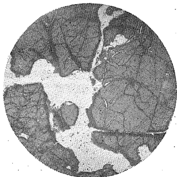
Fig.6 Disseminated chromite with black margin and cross cutting black line. X23 South No.5 deposit of Wakamatsu mine.
