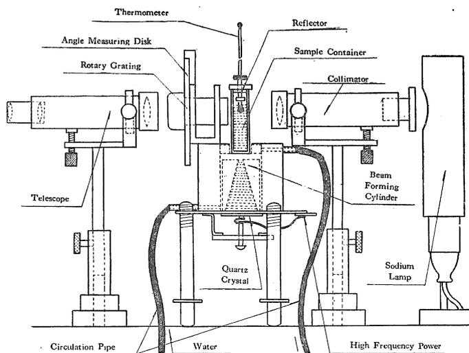
Fig. I Vertical Section of the Experimental Arrangement
