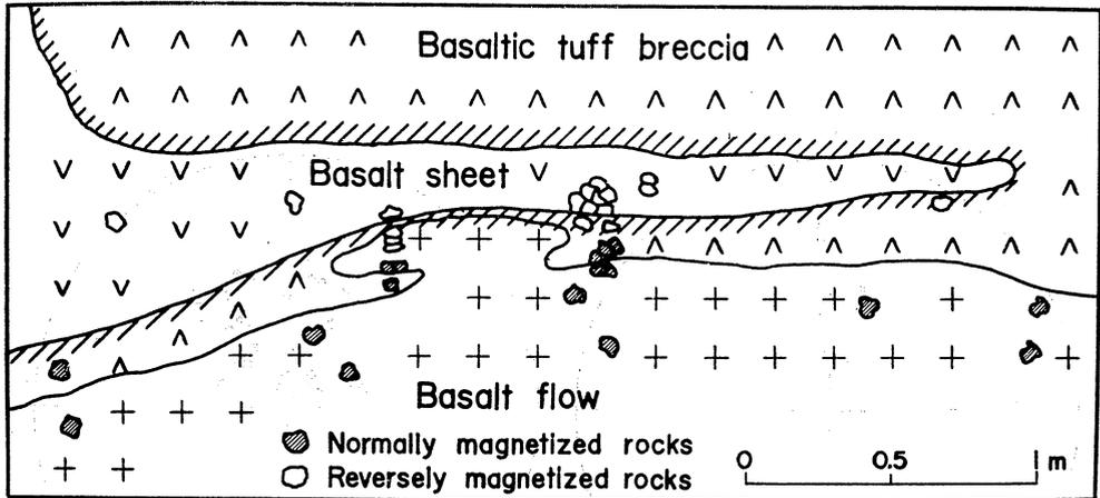
Fig. 6. A typical contact place where baked rock was observed. The shaded portion is metamorphosed rock about 1 cm in thickness.
