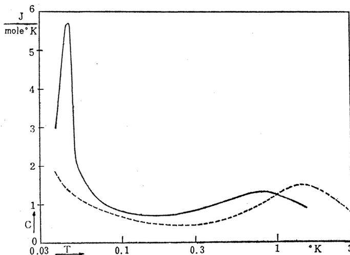
Fig. 3. Comparison of the specific heat versus temperature curves of  $\text{CuSO}_4 \cdot 5\text{H}_2\text{O}$  (dashed line) and  $\text{CuSeO}_4 \cdot 5\text{H}_2\text{O}$  (solid line). The temperatures are plotted on a logarithmic scale. (after Haseda et al.)
