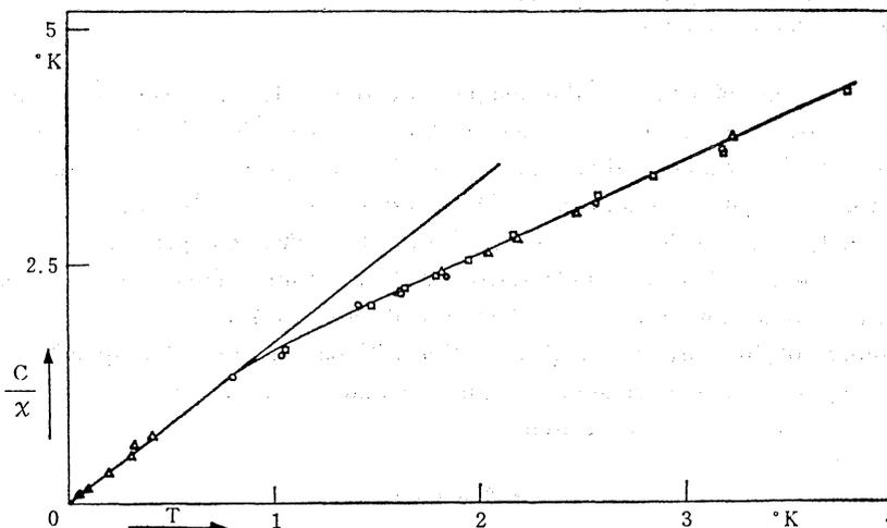
Fig. 2. The ratio of the Curie constant  $C$  and the adiabatic susceptibility  $\chi$  of  $\text{CuSO}_4 \cdot 5\text{H}_2\text{O}$  plotted as a function of temperature below 4°K. (after Haseda et al.)
