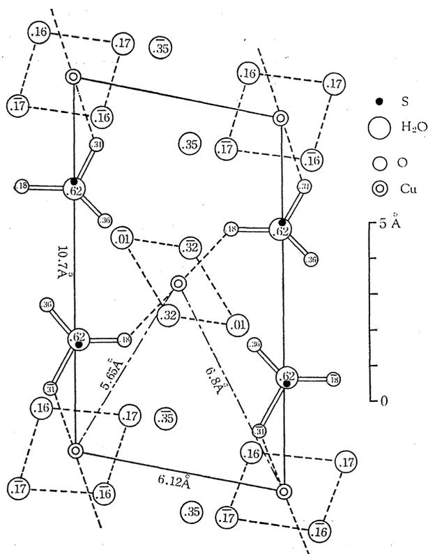
Fig. 1. Projection of the crystal structure of copper sulphate pentahydrate on a plane normal to the  $c$  axis (after Beevers and Lipson). The distances to the plane of the drawing are given in percentages of  $c_0 = 5.97$  Å. The dashed lines between the various oxygen atoms are drawn to show the tetragonal environments of the  $\text{Cu}^{2+}$  ions; the dashed line connecting two oxygens belonging to sulphate groups correspond to the crystal field axes.
