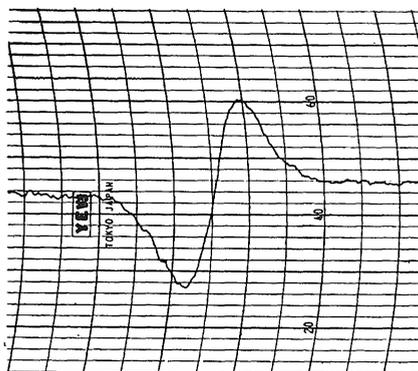
Photo 6 The details of the resonance curve of iodine nuclei in the mixture of iodine and paraffin.
