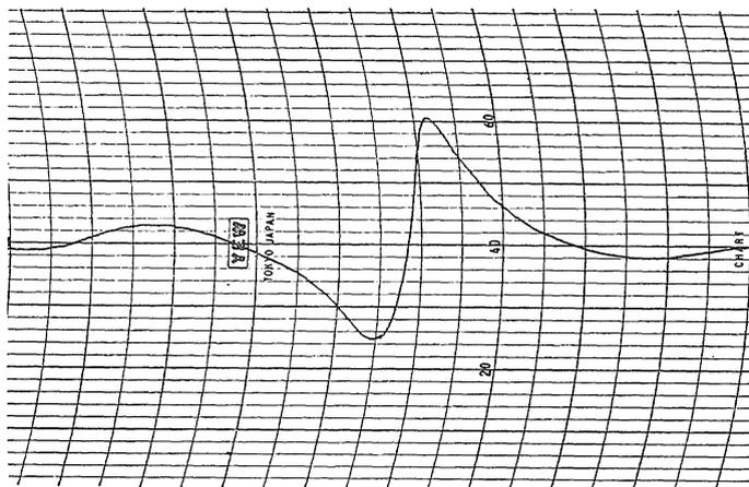
Photo 5 The resonance curve of wave meter.
