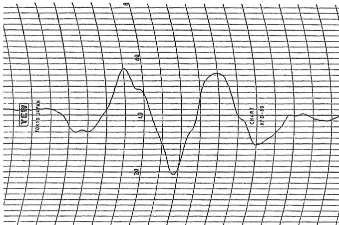
Photo 4 The resonance curve of iodine nuclei in the crystalline state.
