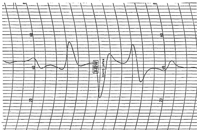
Photo 1 The resonance curve of iodine nuclei in the mixture of iodine and paraffin.
