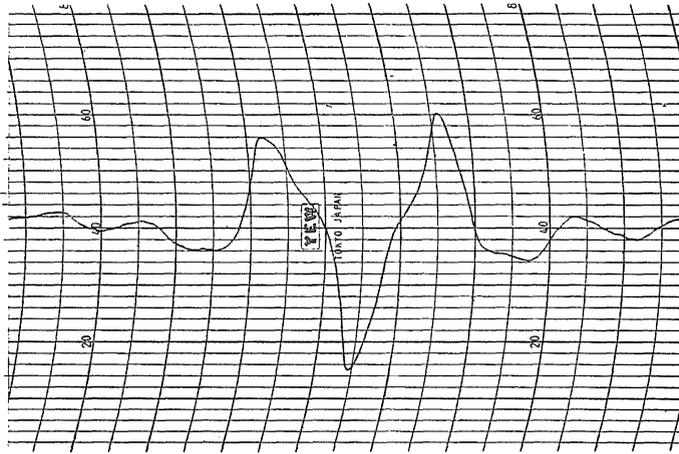
Photo 2 The resonance curve of iodine nuclei in the mixture of iodine and sulfur.
