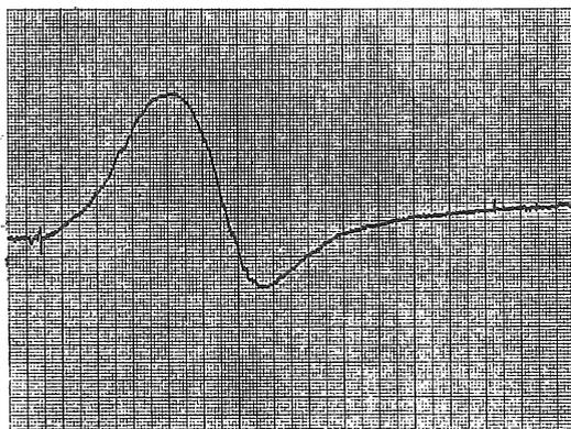
Fig. 2 (c). Derivative curve of resonance line in the irradiated mixture of iodine and paraffin.
