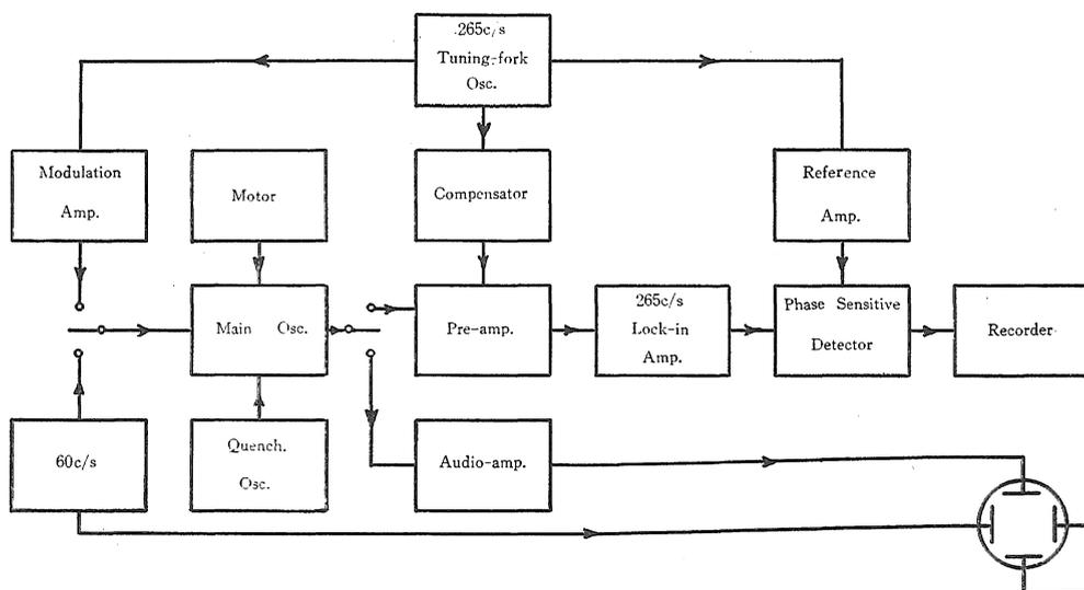
Fig. 1. Block diagram of apparatus.
