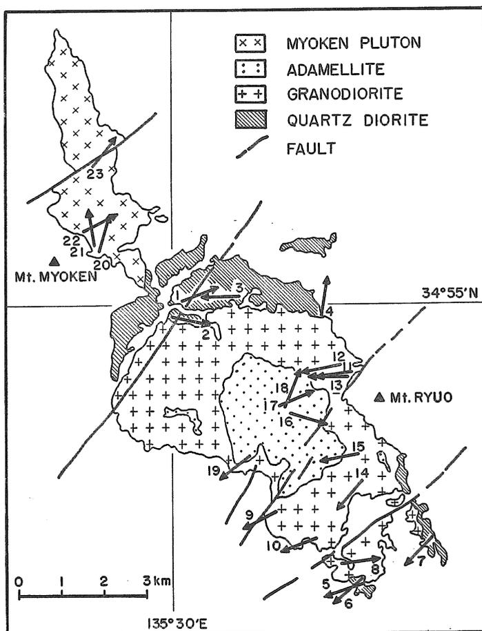
Fig. 3. Declinations of NRM at each sampling site.
