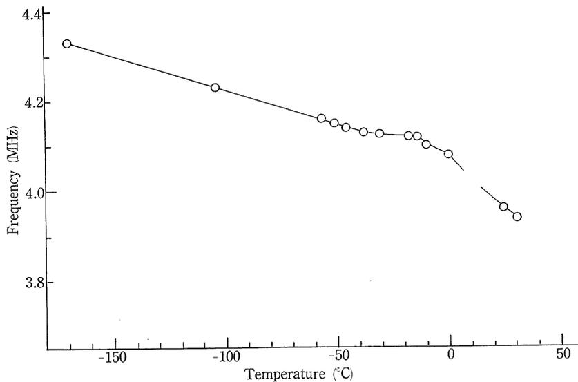
Fig. 4 Dependence of resonance frequency on temperature. The sample is the single crystal whose dimension is about  $1.7 \times 3.6 \times 11 \text{mm}^3$ .
