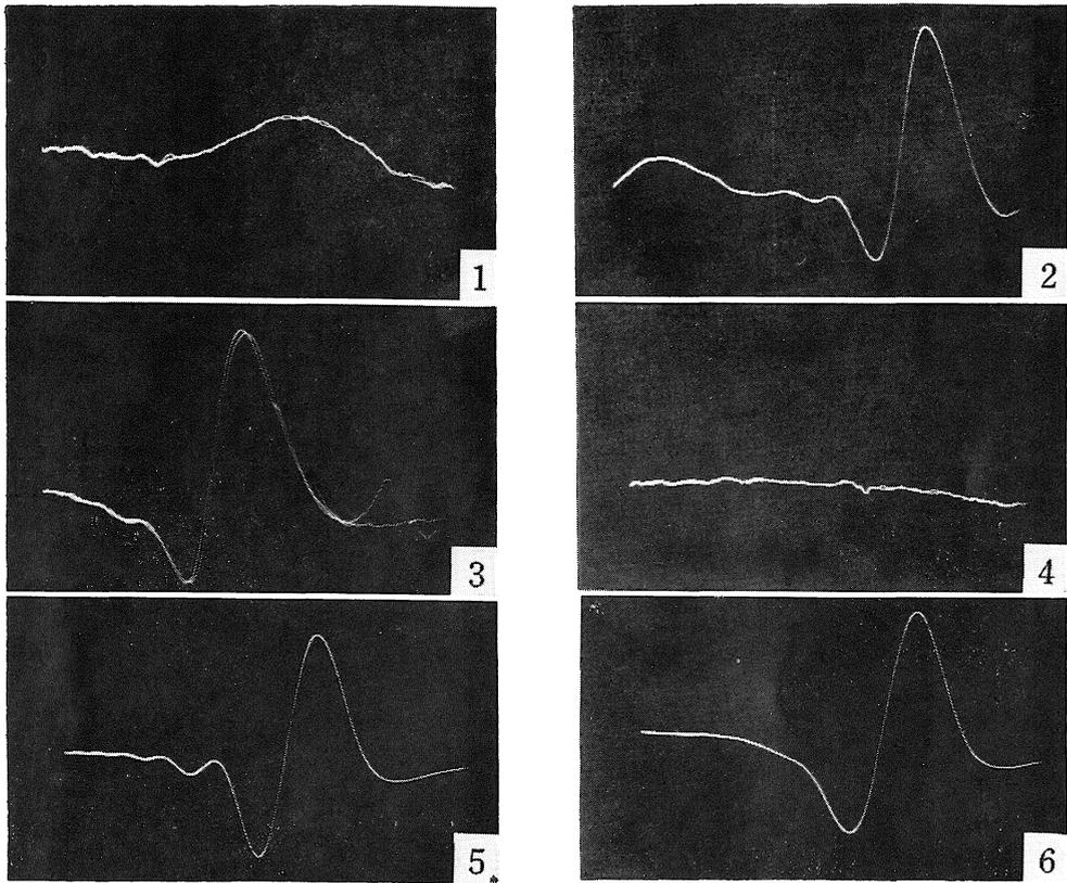
Fig. 6 The absorption lines in quartz resonators observed by a cathode-ray oscilloscope.
