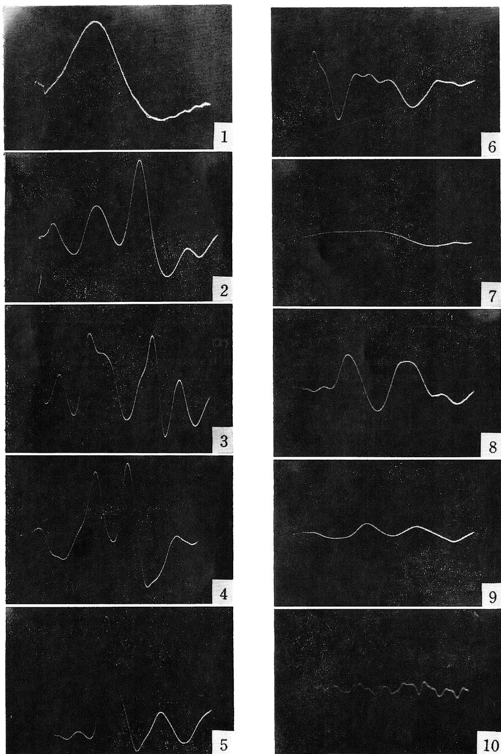
Fig. 3 The absorption lines in pure Rochelle salt observed by a cathode-ray oscilloscope.
