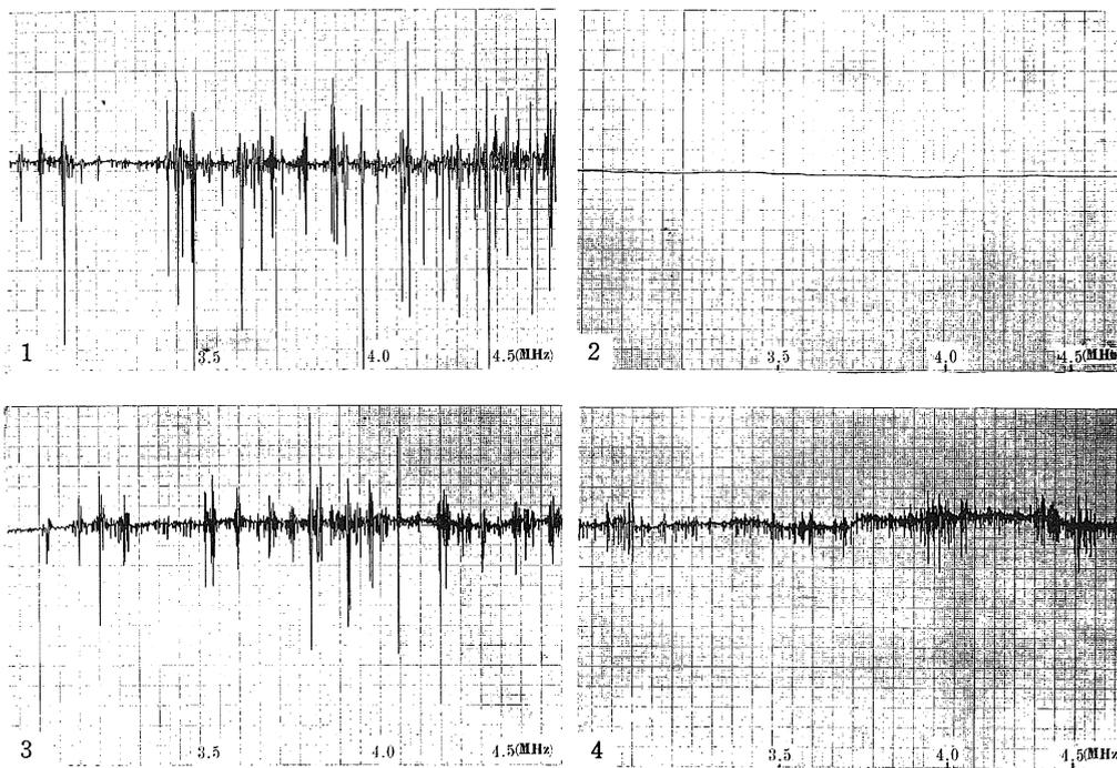
Fig. 5 The pattern of absorption lines recorded by the recorder, in pure Rochelle salt.
