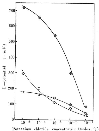
Fig. 2 The effects of potassium chloride on  $\zeta$ -potential of cotton in 0.1018g/l solution of NaPAA-3.
