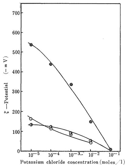
Fig. 3. The effects of potassium chloride on  $\zeta$ -potential of cotton in 0.0512g/l solution of NaPAA-3.
