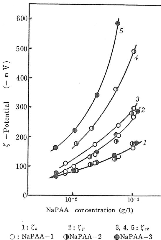
Fig. 1  $\zeta$ -potential of cotton in NaPAA solutions containing  $1 \times 10^{-5}$  moles/l potassium chloride.
