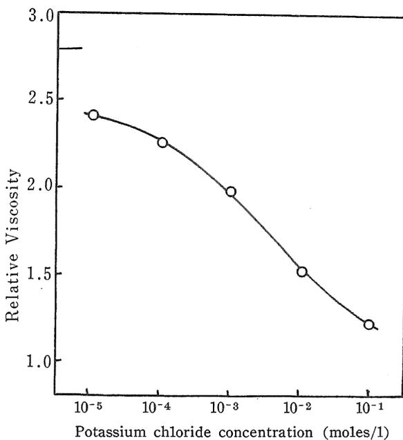
Fig. 4. Plots of viscosity of NaPAA-3 solution against potassium chloride concentration.
