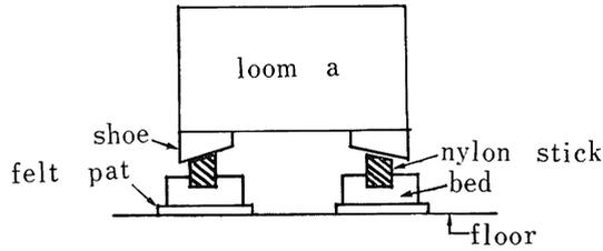
Fig. 7 Loom a and isolator  $\alpha$
