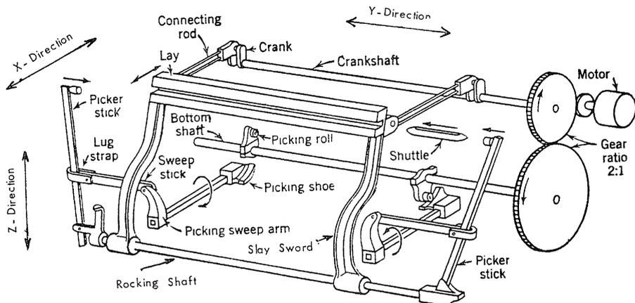
Fig. 2 Schematic diagram of cloth-weaving loom showing principal features that cause shock and vibration
