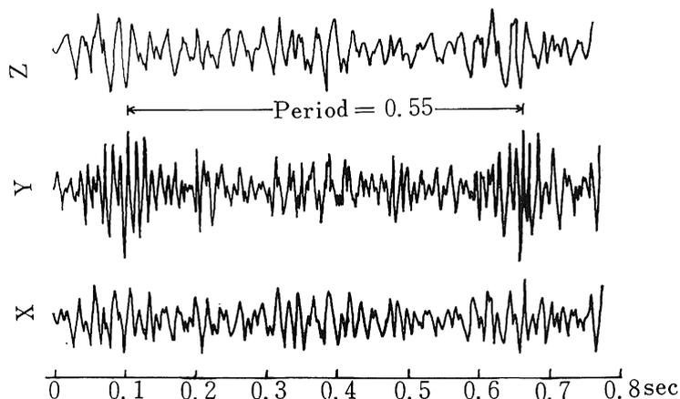
Fig. 10 Acceleration-time Cures. for combination (aA)
