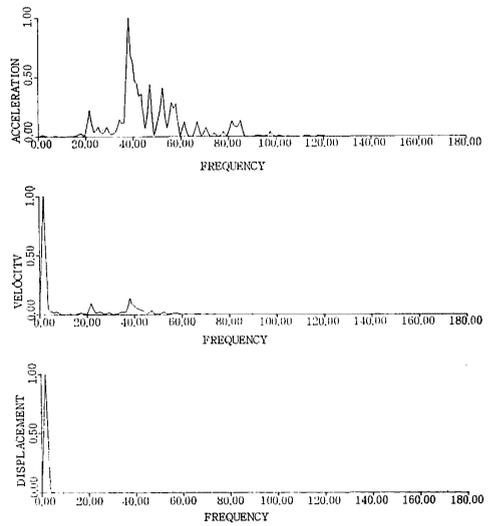
Fig. 14-2 Power spectral density for looms "b" and "b'"
