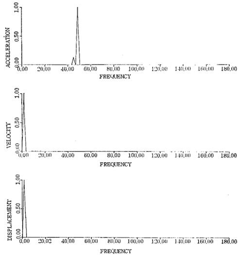
Fig. 14-1 Power spectral density for looms "b" and "b''
