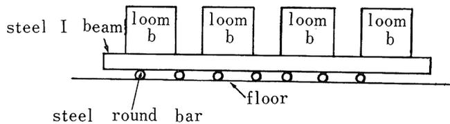
Fig. 9 Looms b and isolator  $\beta$
