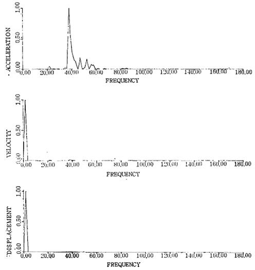
Fig. 14-3 Power spectral density for looms "b" and "b'"
