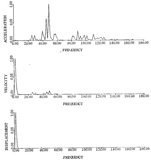
Fig. 13-2 Power spectral density for loom "a" and "a'"
