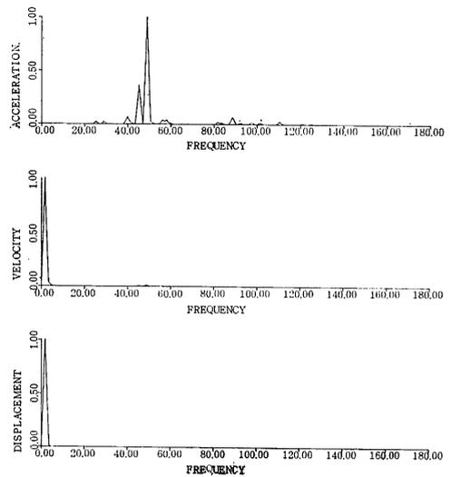
Fig. 13-3 Power spectral density for loom "a" and "a''
