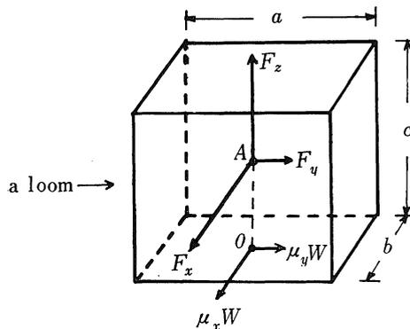
Fig. 3 Reaction forces  $F_x, F_y, F_z$  acting on a loom, and friction forces  $\mu_x W, \mu_y W$  acting on the floor
