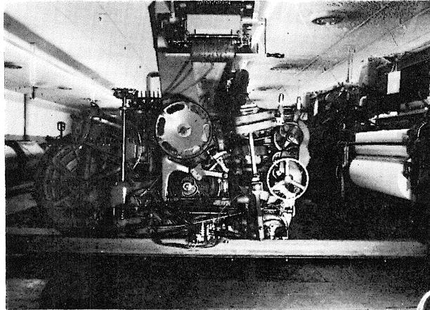
Fig. 8 Looms "b" mounted on the isolator  $\beta$
