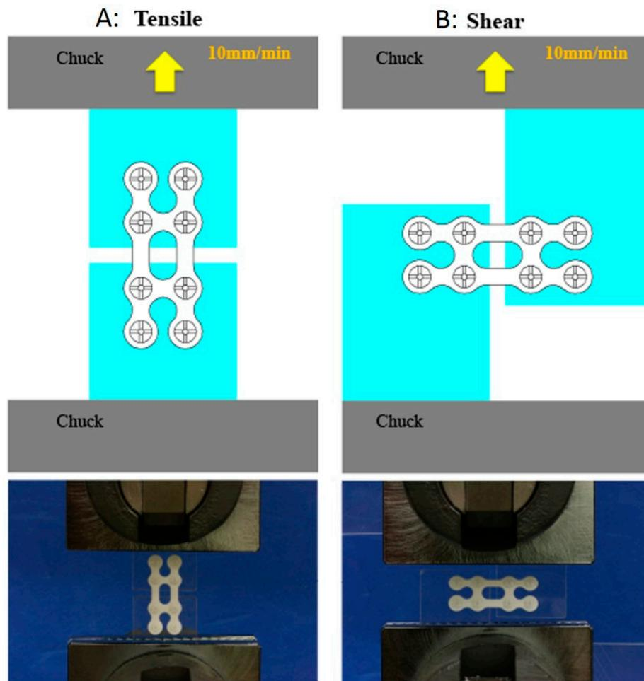
**Figure 1.** Mechanical strength models were prepared by fixing the plate with screws to the polycarbonate plate. (A). Tensile strength; (B). Shear strength.
