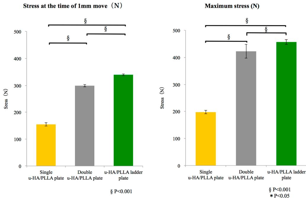
**Figure 4.** Mean values and respective standard deviations for the tensile strength test for each group. Left graph shows the maximum stress, and the right graph shows the stress during 1-mm movement in tensile strength.
