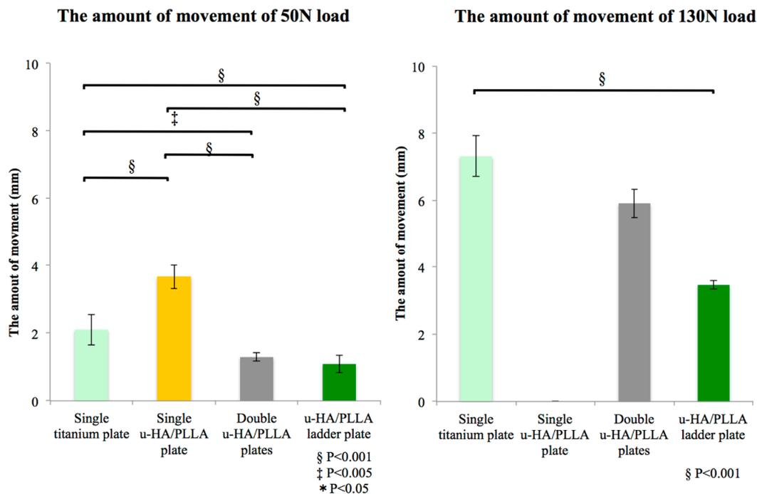
**Figure 6.** Mean values and respective standard deviations for the amount of movement by adding load for each group. Left graph shows the amount of movement with 50 N load, and the right graph shows the amount of movement with 130 N load.
