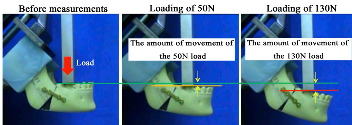
**Figure 3.** A linear load in the mandibular first molar region was applied at a displacement speed of 10 mm/min. We compared the amount of movement at the time of the load in the postoperative average occlusal force (postoperative 1 week, about 50 N, and postoperative 1 month, about 130 N) to the reference.
