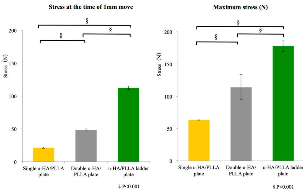
**Figure 5.** Mean values and respective standard deviations for the shear strength test for each group. Left graph shows the maximum stress, and the right graph shows the stress during 1-mm movement in shear strength.
