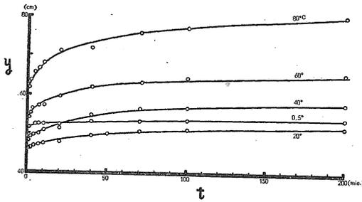
Fig. 2. Examples of original creep curves at different temperatures.
