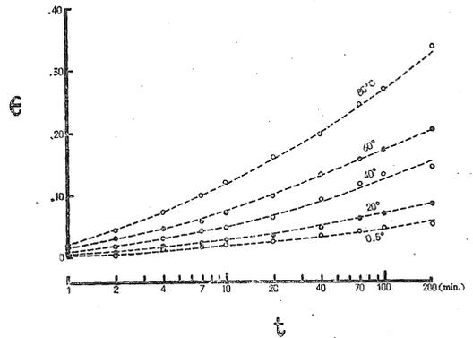
Fig. 4. Creep curves shown by  $\epsilon - \log t$  at different temperatures.
