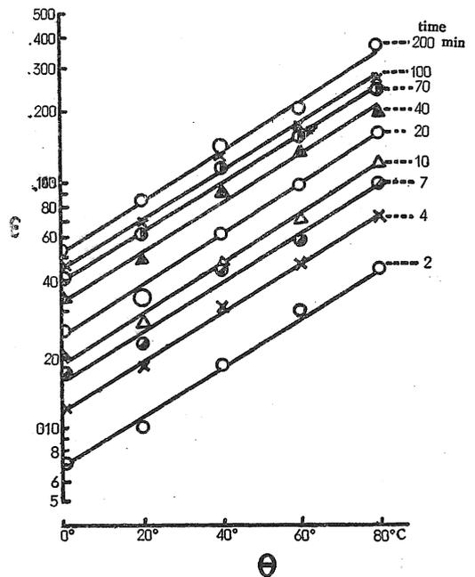
Fig. 7 Relationship between  $\log \epsilon$  and temperature at different times.
