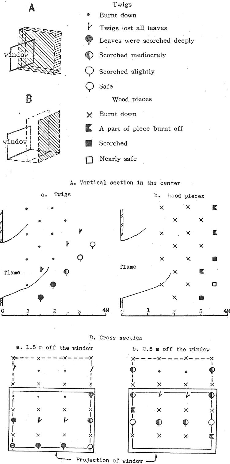
Fig. 8. Fire resistance of leaves in front of a window.
