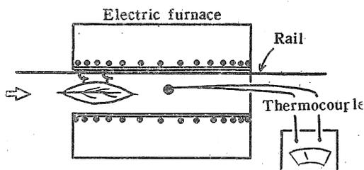
he carried comparative tests of trees on (1) the flashing types, (2) flammabilities and (3) the time required for flashing, among leaves of 74 species of common tree in Japan.
