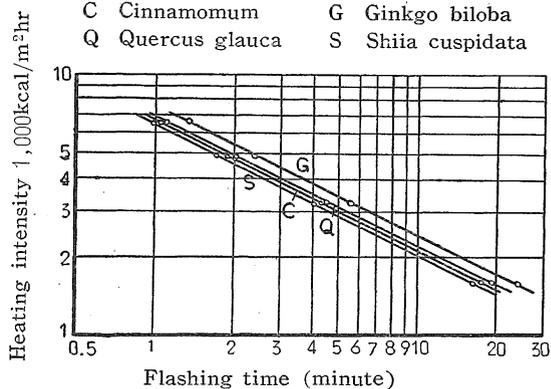
2. Flashing time tests in a small scale (by a electric furnace)
