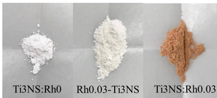
Figure 4.1 Picture of synthesized non-doped Ti3NS (Ti3NS:Rh0), Rh-loading Ti3NS (Rh0.03-Ti3NS), and Rh-doping Ti3NS (Ti3NS:Rh0.03).
