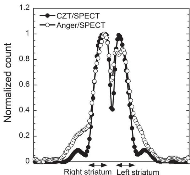
Fig. 3. Count profile curve for the bilateral caudate nuclei. Better image contrast between the striatum and the background region was seen on the cadmium-zinc-telluride (CZT)/SPECT scan than on the Anger/SPECT scan. The CZT/SPECT scan displayed an approximately 41 times higher peak count (2738 counts) than the Anger/SPECT scan (66 counts).
