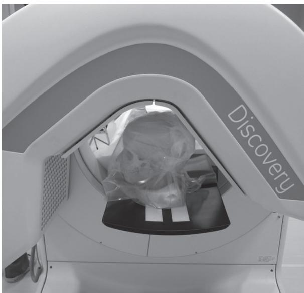
Fig. 1. Phantom setup for the cadmium-zinc-telluride (CZT)/SPECT scan. The phantom was scanned in a seated position using CZT/SPECT for 5 min. The sagittal plane of the phantom ran perpendicular to the gantry axis.
