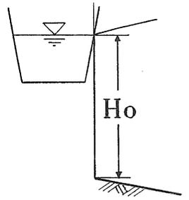
Fig 3 Boundary condition : groundwater table  $z_1 = H_0$  at  $x=0$
