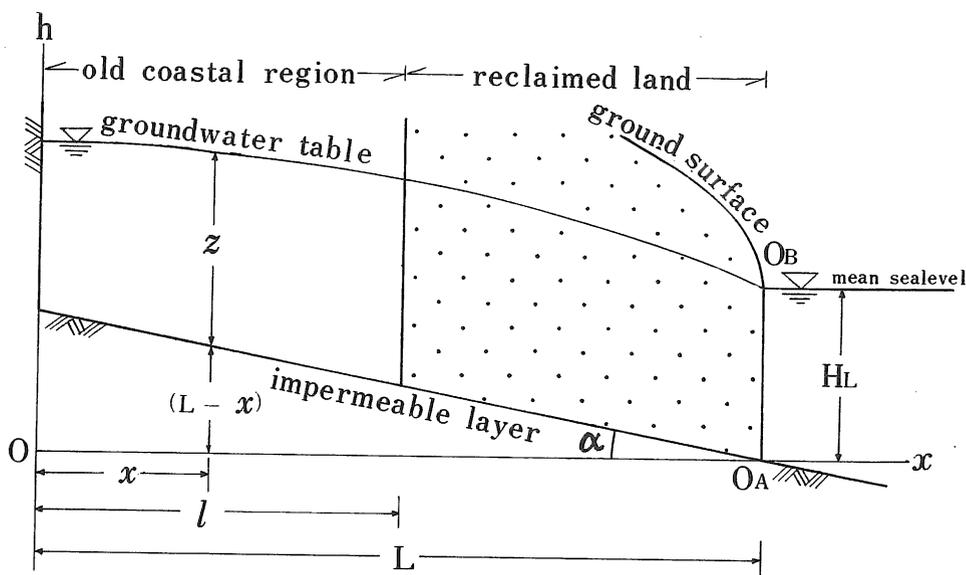
Fig 1 Diagrammatic representation of the groundwater table in the coastal region
