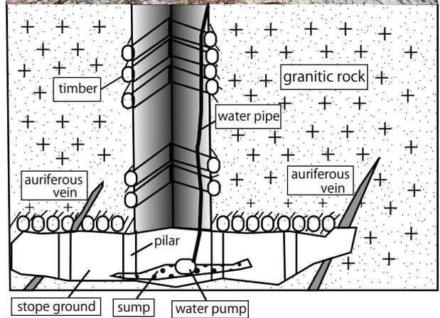
**Fig. 3** Photo and sketch indicating shaft for excavation of gold and auriferous ore bearing material at Nzunguni gold mining (Madengi Hill) in central Tanzania. Shaft was constructed vertically and the soft walls were protected by timbers. Stope ground was formed underground of which was supported by timber pillars and to drain the sump (water pit) by water pump. White material around the shaft is drained weathered rocks.
