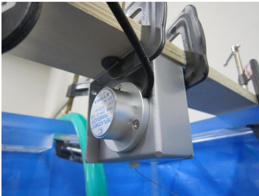
**Figure 4.4** Location of the linear displacement transducer inside the flume tank.
