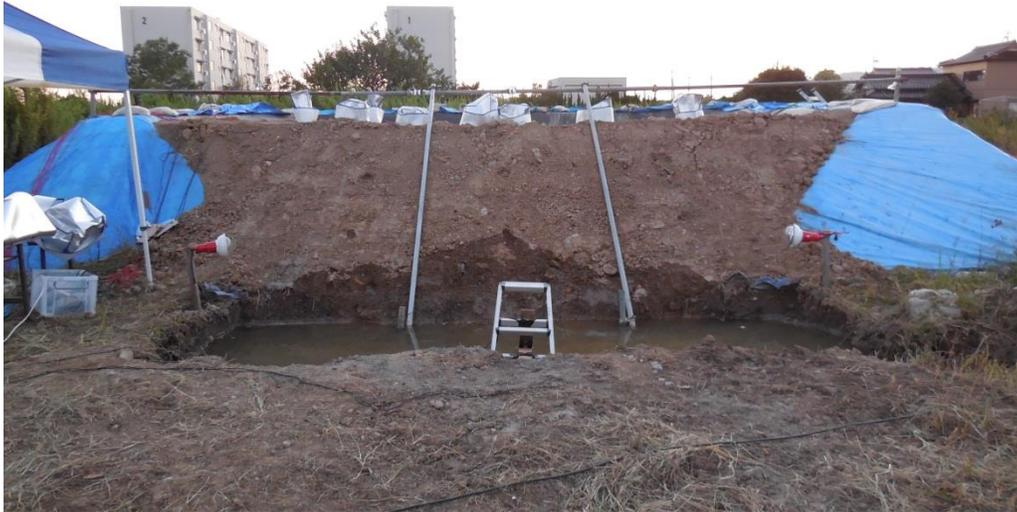
**Figure 7.8** Gradual unraveling of the downstream toe under steady-state saturation.
