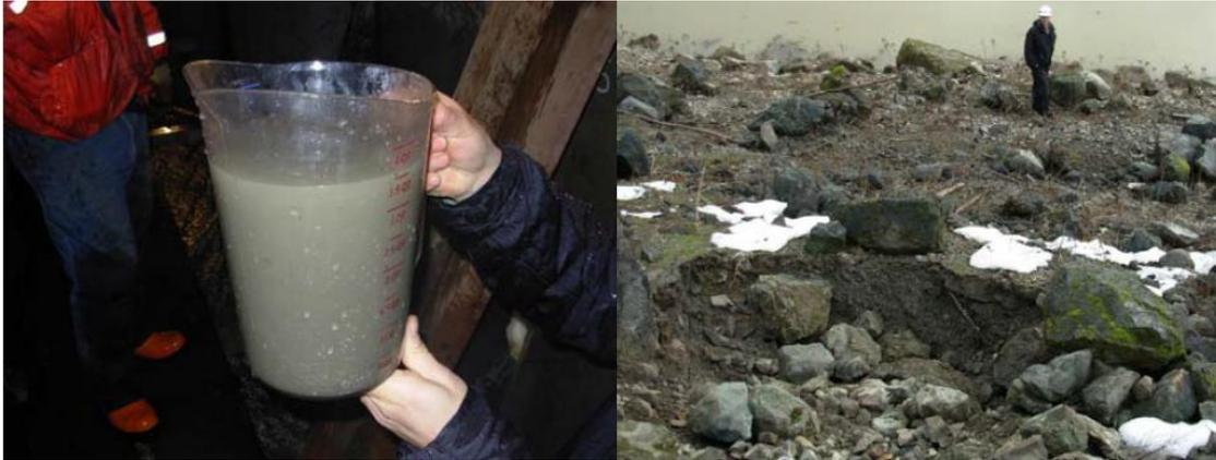
**Figure 7.17** Investigation of seepage in Howard Hanson Dam, USA. (a) Turbid water collected from a vertical drain at the right abutment, (b) Occurrence of a large depression at the upstream slope of the right abutment.
