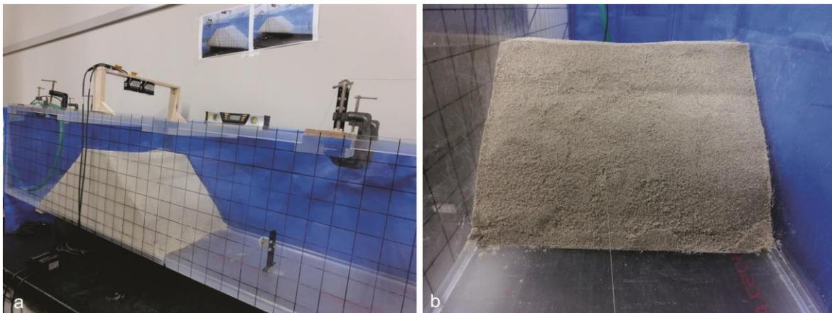
**Figure 4.10** **a** Side view of the flume tank. **b** Front view of a dam showing the downstream slope prior to commencement of an experiment.
